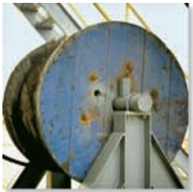
Unwinding the cable from this spool requires overcoming friction from the supporting shaft. (© Russell C. Hibbeler)
