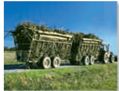
During high winds and when going around a curve, these sugar-cane trucks can become unstable and tip over since their center of gravity is high off the road when they are fully loaded. (© Russell C. Hibbeler)
