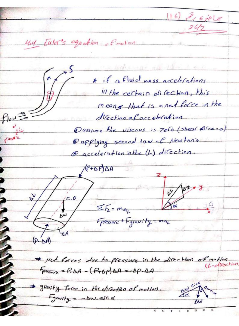
EF\_ = may = Fressure + Fgravity = may L> - DP. DA - DWSin X = MAL where D DW=M.g DW=P.V.g \_\_ DW=P.DA.AL.g @ Sink = AZ 3 m= g. DA. DL DP-DA-PDADLY . DZ = (P.DA.DL)QL / DA.DL LE SPARSANIZATE - OP - 8 - AZ - P. az - take the limit to Al-so
