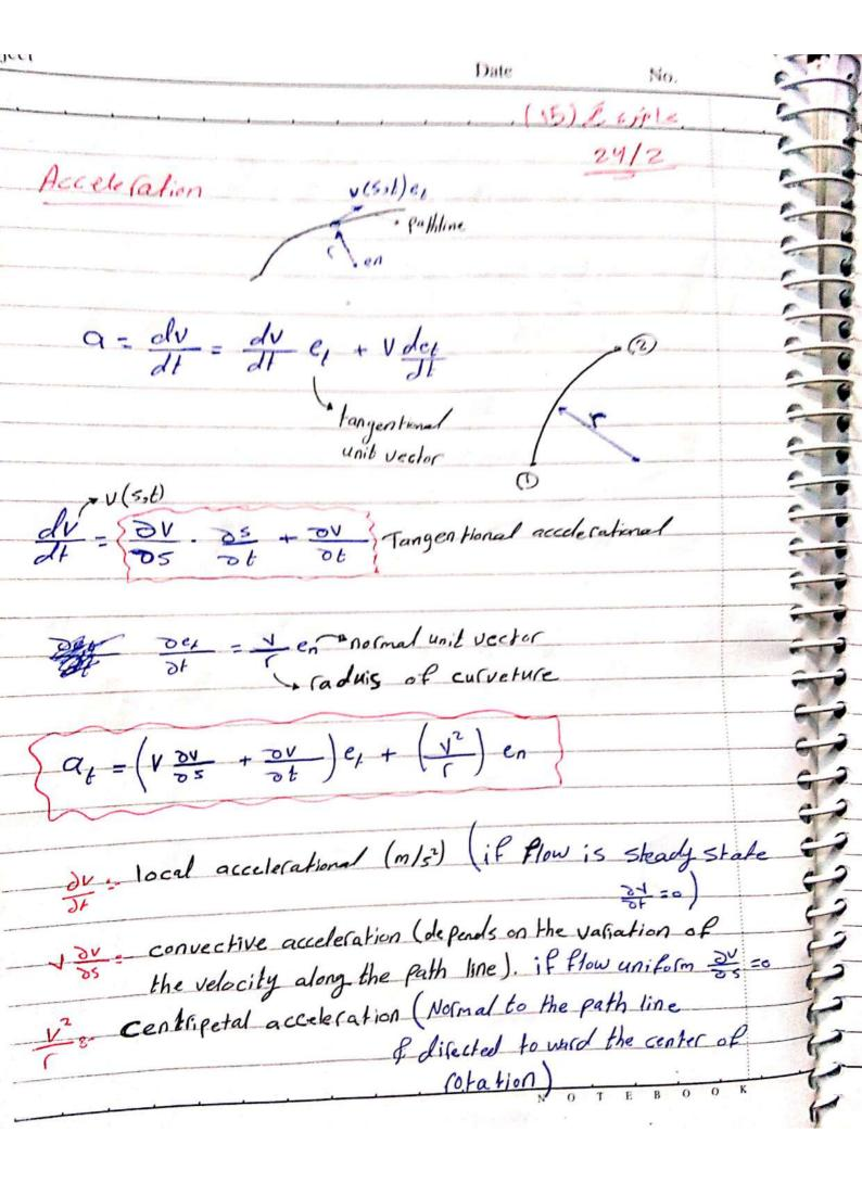
abject The velocity along the pathline is given by V(s,t) = 3 t/2, the raduis of curvature is 0.5m, Evalute the acceleration long & normal to the pathline at  $\frac{\partial u}{\partial t} + \frac{\partial v}{\partial t} \right) e_t + \frac{v^2}{\Gamma} e_n$ , at  $\frac{d}{dt} = 2m$ 2 \*2 \* 0.5 = 2.828m/s # =0.5 t=0.5 2.828 x 2.828 + 2.828)ex +16en -10.82ex +16en
