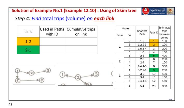
Solution of Example No.1 (Example 12.10) : Using of Skim tree الجامعين الجاشينين ( Step 4: Find total trips (volume) on each link Estimated Used in Paths Cumulative trips Nodes Link Shortest trips Path ID with ID on link Path between From То zones =100+100=200 2 1-2 100 1-2 1 and 2 1 3 1-2,2-3 2 100 1 1-5,5-4 4 3 200 =400+200=600 2-1 5 and 9 5 1-5 4 150 1 2-1 400 2-3 3 6 200 .3 2 4 2-4 100 7 5 2-4,4-5 8 500 1 3-2,2-1 9 200 2 3-2 10 100 3 4 3-4 11 100 3-4,4-5 5 12 150 4 5-4 20 350
