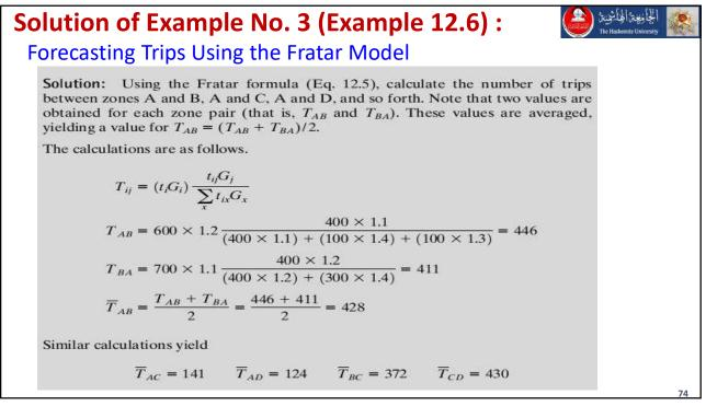
$$T_{AB} = (t_A G_A)_{+} \frac{t_{AB} G_B}{\sum_{z=0}^{N-D} t_{AB} G_A}$$
