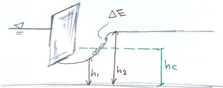
$$\checkmark \frac{h_1^2}{2} + \frac{q_1^2}{gh_1} = \frac{h_2^2}{2} + \frac{q_2^2}{gh_2} \quad > \text{Rect.}$$
