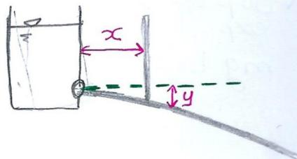
\* Part I: Coefficient of velocity - (C<sub>v</sub>)
