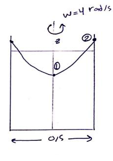
$$\frac{P_{1}}{8} + \frac{2}{1} - \frac{\omega^{2} r_{1}^{2}}{29} = \frac{P_{2}}{8} + \frac{2}{2} - \frac{\omega^{2} r_{2}^{2}}{29}$$
