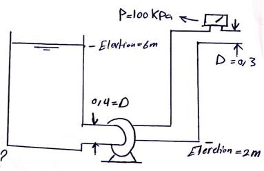
$$\frac{P_{1}}{8} + \frac{V_{1}^{2}}{2g} + Z_{1} + h_{P} = \frac{P_{2}}{8} + \frac{V_{2}V_{2}^{2}}{2g} + Z_{2} + h_{F} + h_{L}$$
