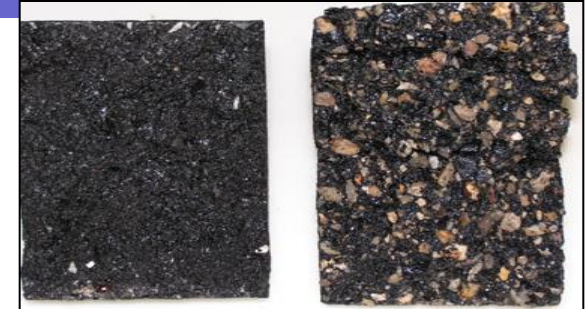
Samples with no moisture damage (left) and moisture damage (right). Notice the amount of uncoated aggregate on the damaged sample.
