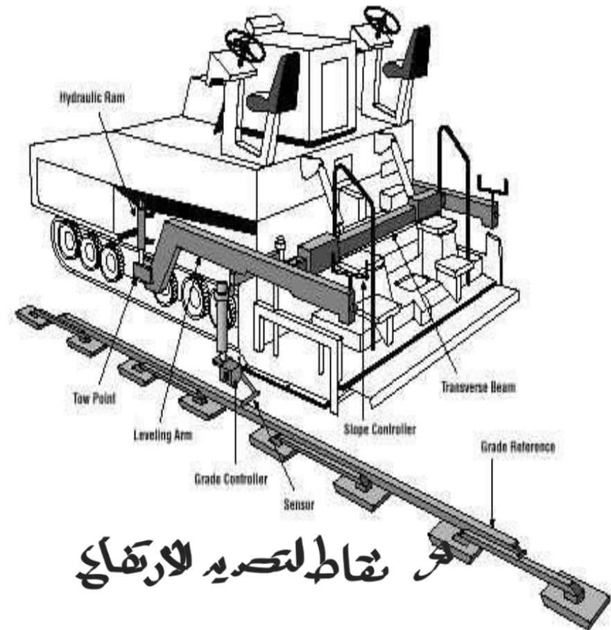
Figure 5.17 Automatic Screed Reference System
