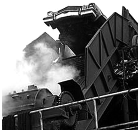
FIGURE 6.8 Auto entering shredder. (Reproduced with kind permission of Sims Group Limited, Cadillac Faces Shredder Jaws , n.d. Available from: http://www.unitednotions.com.au/prjob_7.html .)
