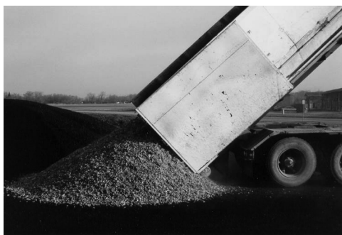
FIGURE 9.16 Piles of coal and RDF to be mixed in the field prior to shipment to heating plant.
