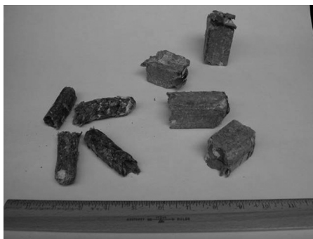
FIGURE 9.15 Two types of densified RDF: pellets and cubettes.
