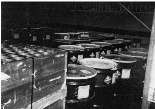
FIGURE 12.3 Aisle space must be sufficient to allow the movement of persons and equipment. (This facility is not in compliance.)
