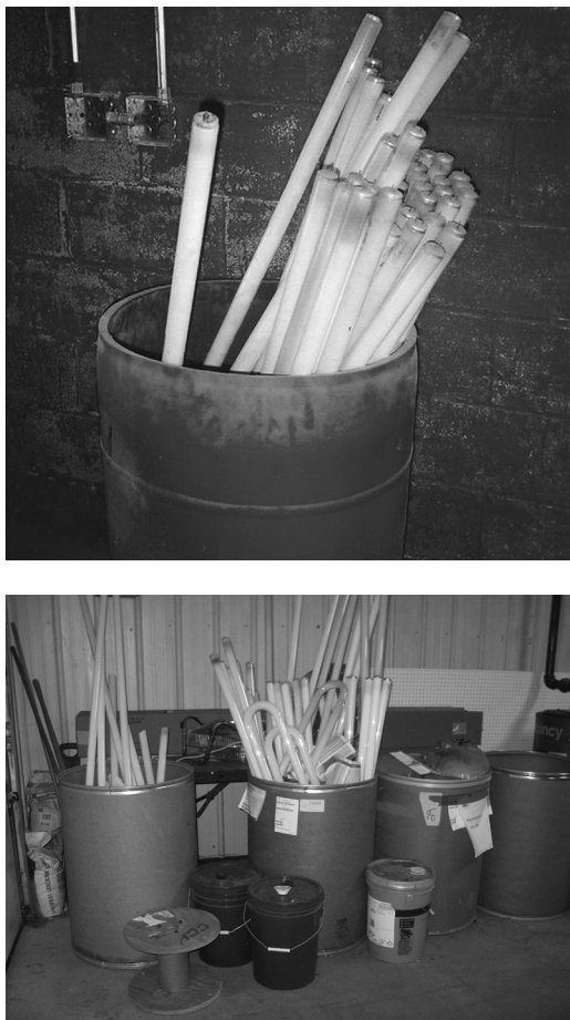
FIGURE 18.1 Clearly not the proper method to manage universal waste lamps.
