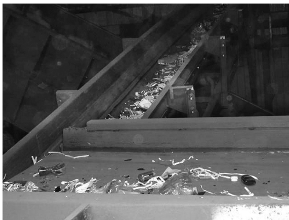
FIGURE 7.7 Transfer point along a conveyor belt. Wastes sometimes fall away from the belts during transfer to another belt.
