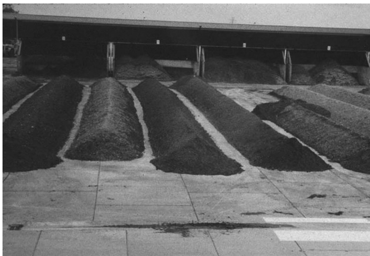
FIGURE 8.5 Composting of MSW by using the windrow system.
