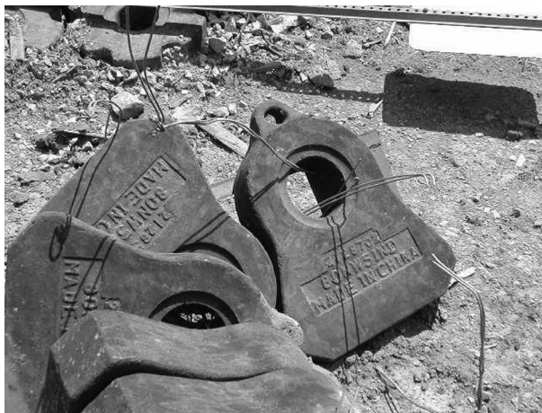
FIGURE 7.22 A new hammer for a horizontal hammermill.
