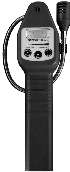
FIGURE 10.15 Portable organic vapor analyzer. (From Federal Emergency Management Agency, Landfill Fires. Their Magnitude, Characteristics, and Mitigation , May 2002/FA -225, 2002, Available from: http://www.usfa.fema.gov/downloads/pdf/publications/fa-225.pdf .)
