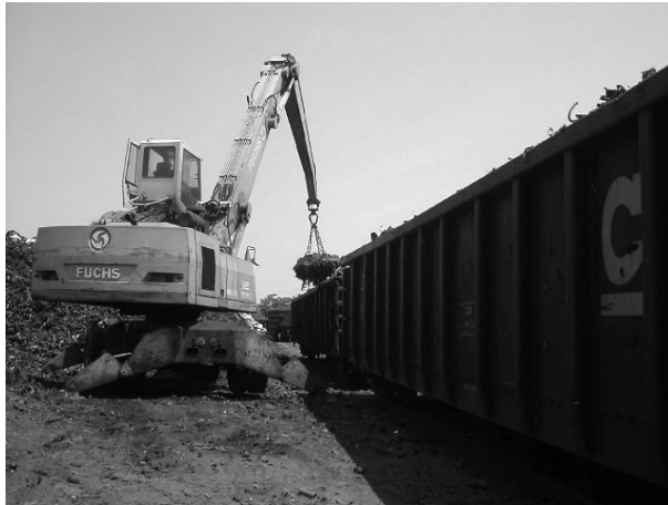
FIGURE 6.9 Electromagnet for moving ferrous wastes onto rail cars.
