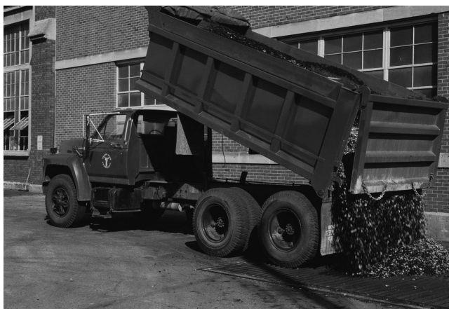
FIGURE 9.17 Truck loading a coal–RDF mixture for combustion at a heating plant.
