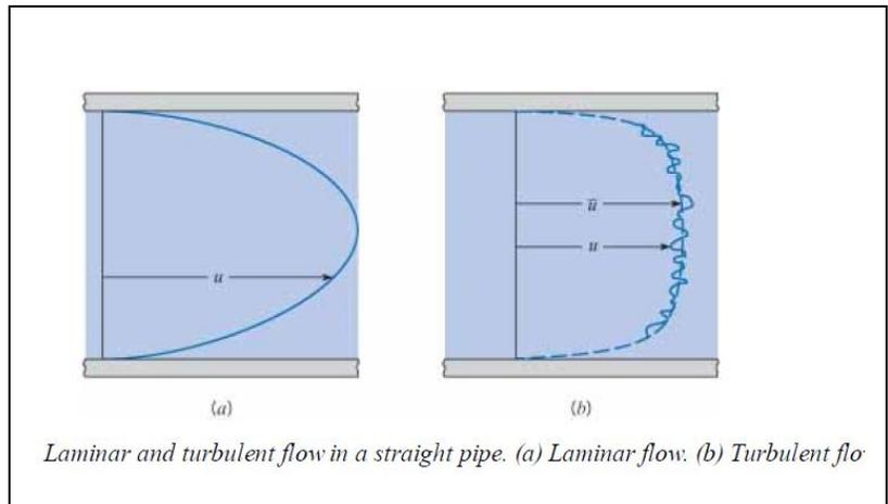
The standard approach to treating turbulent flow is to represent the velocity as a time-averaged average value plus a fluctuating quantity,  $u = \bar{u} + u'$ . The time-averaged value is designated  $\bar{u}$  by in Fig. (b). The fluctuation velocity is the difference between the local velocity and the averaged velocity. A turbulent flow is often designated as “steady” if the time-averaged velocity is unchanging with time.
