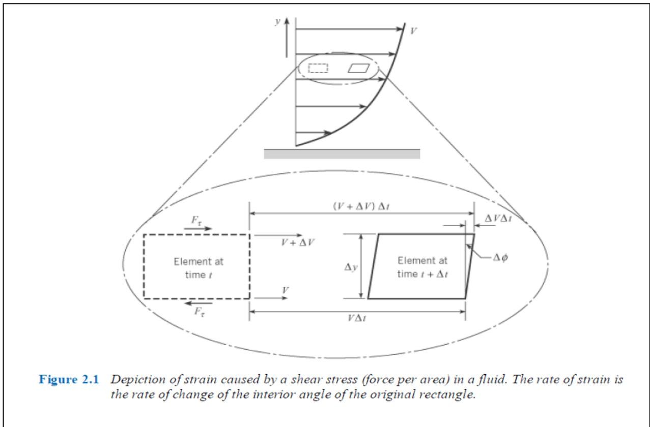
**Figure 2.1** Depiction of strain caused by a shear stress (force per area) in a fluid. The rate of strain is the rate of change of the interior angle of the original rectangle.
