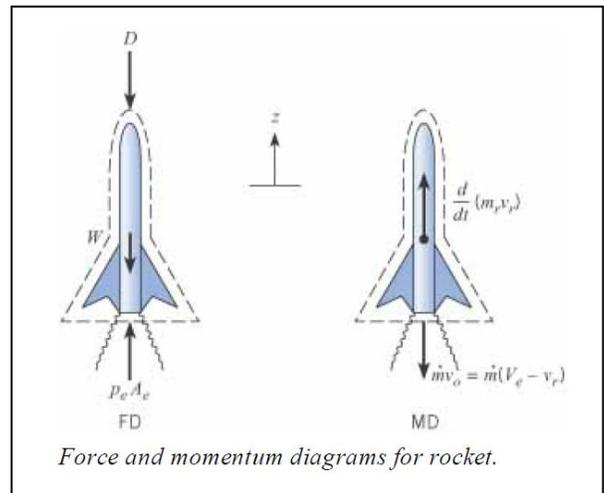
$$v_{bo} = \frac{T}{\dot{m}} \ln \frac{m_i}{m_f}$$
