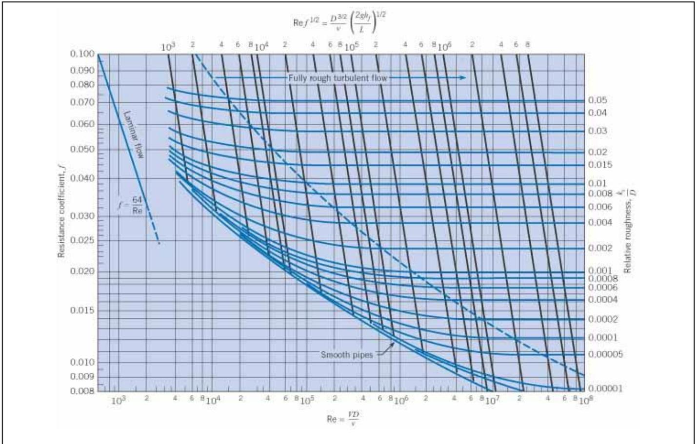
To provide a more convenient solution to some types of problems, the top of the Moody diagram presents a scale based on the parameter  $Re f^{1/2}$ . This parameter is useful when  $h_f$  and  $ks/D$  are known but the velocity  $V$  is not.
