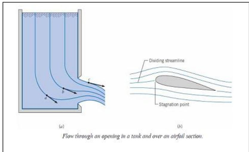
Whenever flow occurs around a body, part of it will go to one side and part to the other as shown in Fig. (b) for flow over an airfoil section. The streamline that follows the flow division (that divides on the upstream side and joins again on the downstream side) is called the *dividing streamline*. At the location where the dividing streamline intersects the body, the velocity will be zero with respect to the body. This is the *stagnation point*.
