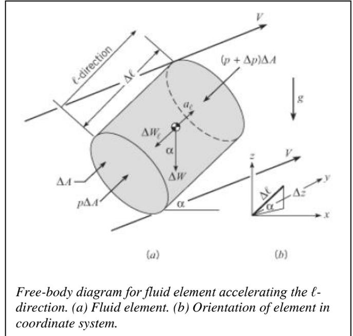
Free-body diagram for fluid element accelerating the  $\ell$ -direction. (a) Fluid element. (b) Orientation of element in coordinate system.
