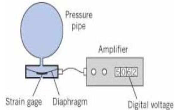
*Schematic diagram of strain-gage pressure transducer.*
