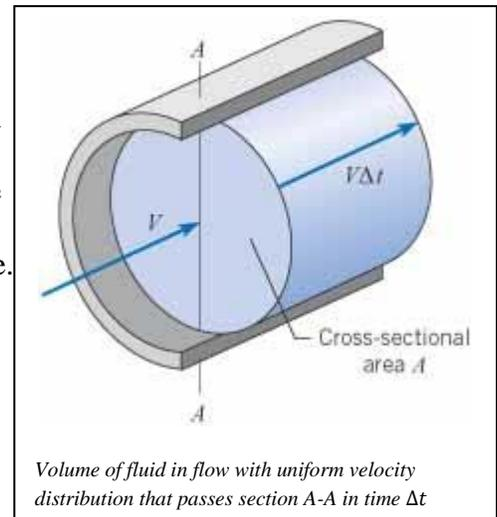
In general, the velocity varies across the section such as shown in Fig. The volume flow rate through a differential area of the section is  $V dA$ , and the total volume flow rate is obtained by integration over the entire cross-section
