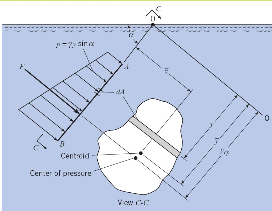
Pressure on the differential area can be computed if the  $y$  distance to the point is known
