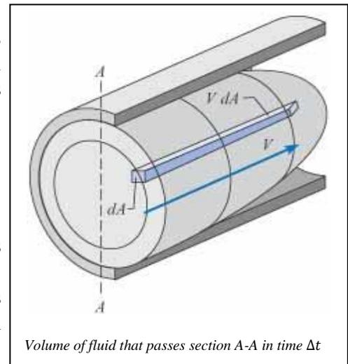
The volume flow rate equation can be generalized by using the concept of the dot product. The flow velocity vector is not normal to the surface but is oriented at an angle  $\theta$  with respect to the direction that is normal to the surface. The only component of velocity that contributes to the flow through the differential area  $dA$  is the component normal to the area,  $V_n$ . The differential discharge through area  $dA$
