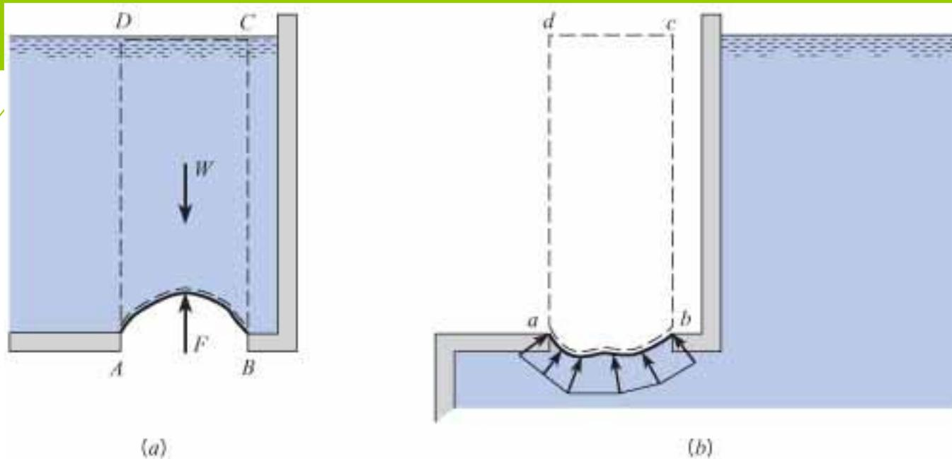
If the region above the surface, volume  $abcd$ , were filled with the same liquid, the pressure acting at each point on the upper surface of  $ab$  would equal the pressure acting at each point on the lower surface. In other words, there would be no net force on the surface
