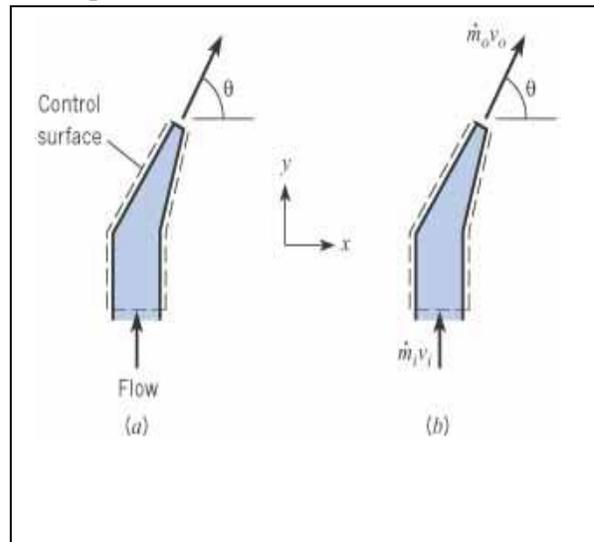
In summary, the momentum of the material inside a control volume is evaluated by integrating the momentum of each volume element over the control volume. If the momentum in each differential volume is constant with time (e.g., steady flow, a stationary structural part), the momentum accumulation rate is zero.
