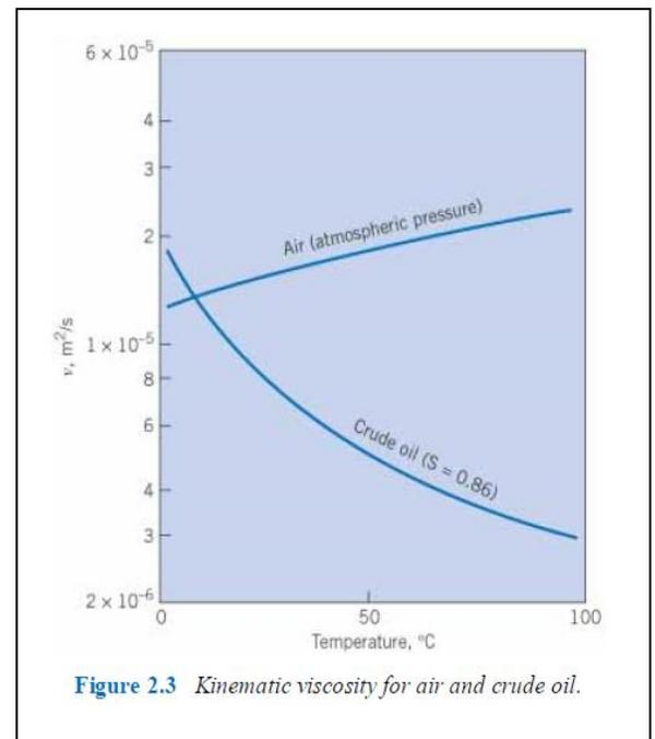
Figure 2.3 Kinematic viscosity for air and crude oil.
