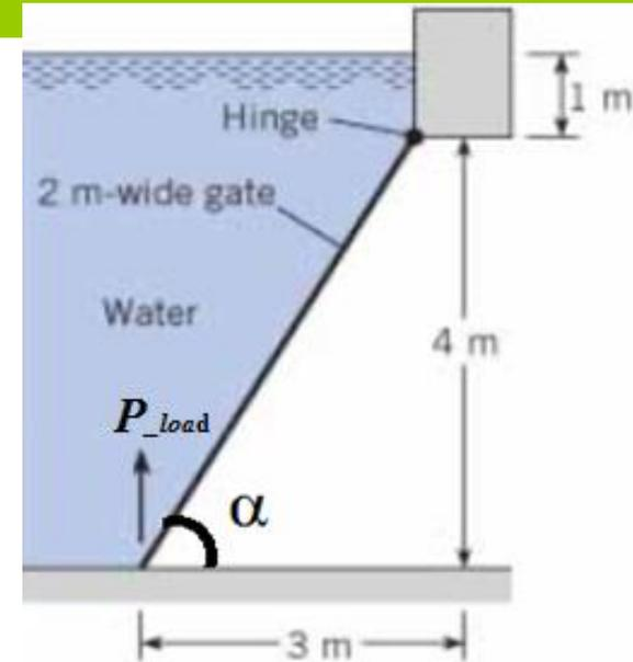
$y_{cp} - \bar{y} = \frac{\bar{I}}{y A}$  where  $\bar{y} = h / \sin \alpha$  : slanted distance from the surface
