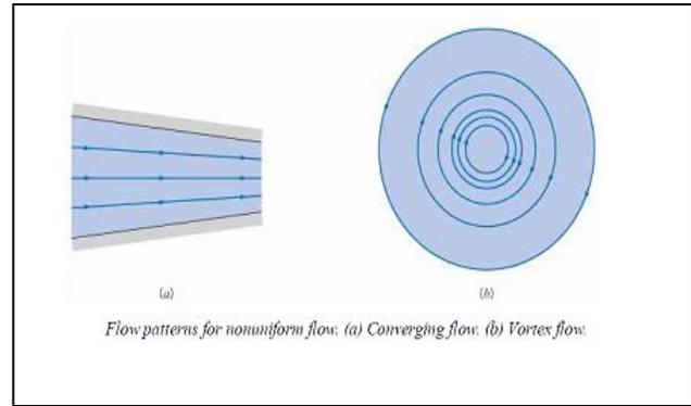
Flows can be either steady or unsteady. In a *steady flow* the velocity at a given point on a fluid path does not change with time:  $\frac{\partial V}{\partial t} = 0$ .
