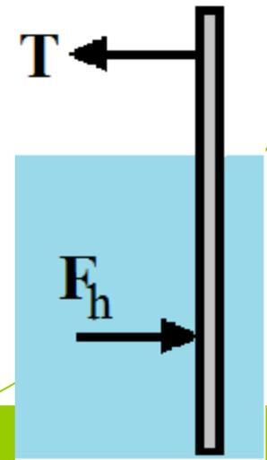
$$T = mg - F_b = \gamma_{block} Vol - \gamma_{water} Vol$$
