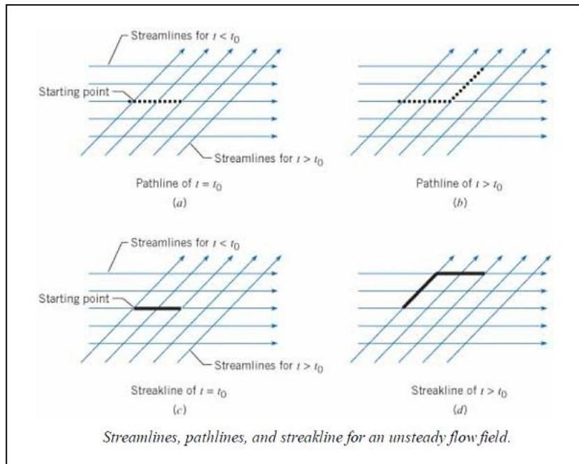
Obviously, the pathline and streakline are very different. In general, neither pathlines nor streaklines represent streamlines in an unsteady flow. Both the pathline and streakline provide a history of the flow field, and the streamlines indicate the current flow pattern.
