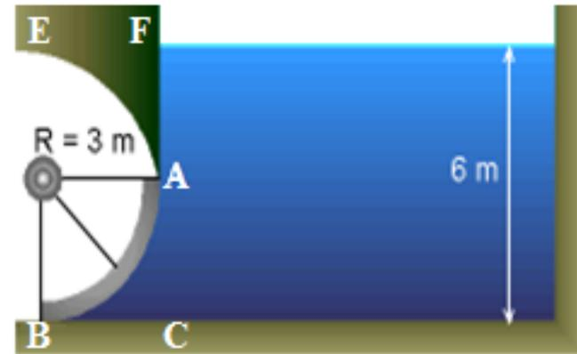
the y-component of the resultant force is the weight of the water directly above the curved surface (i.e., imaginary volume ABEF).
