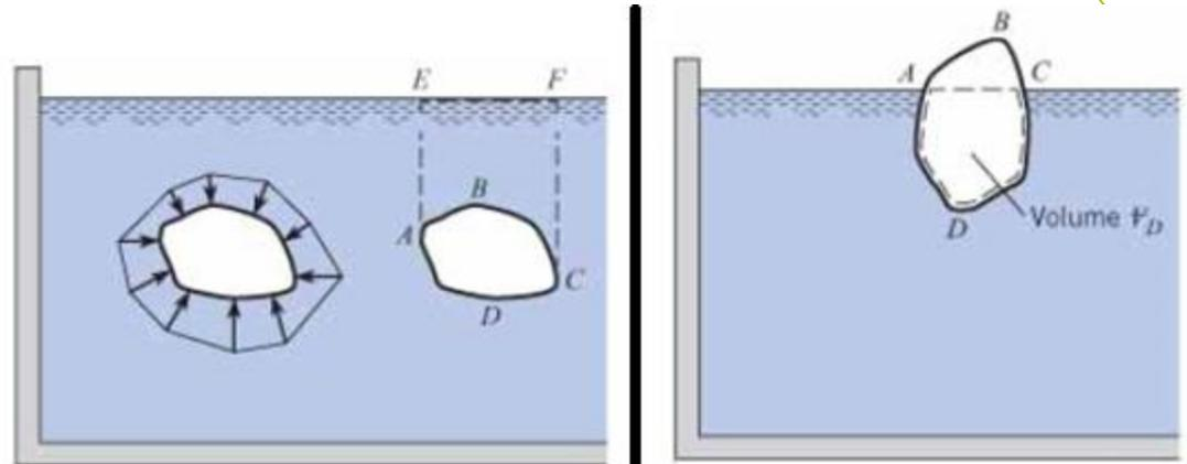
Two views of a body immersed in a liquid. A body partially submerged in a liquid.
