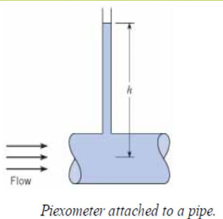
vertical tube-transparent- in which a liquid rises in response to a positive gage pressure.
