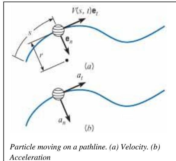
where  $V(s, t)$  is the speed of the particle, which can vary with distance along the pathline,  $s$ , and time,  $t$ . The direction of the velocity vector is given by a unit vector  $\mathbf{e}_t$ .
