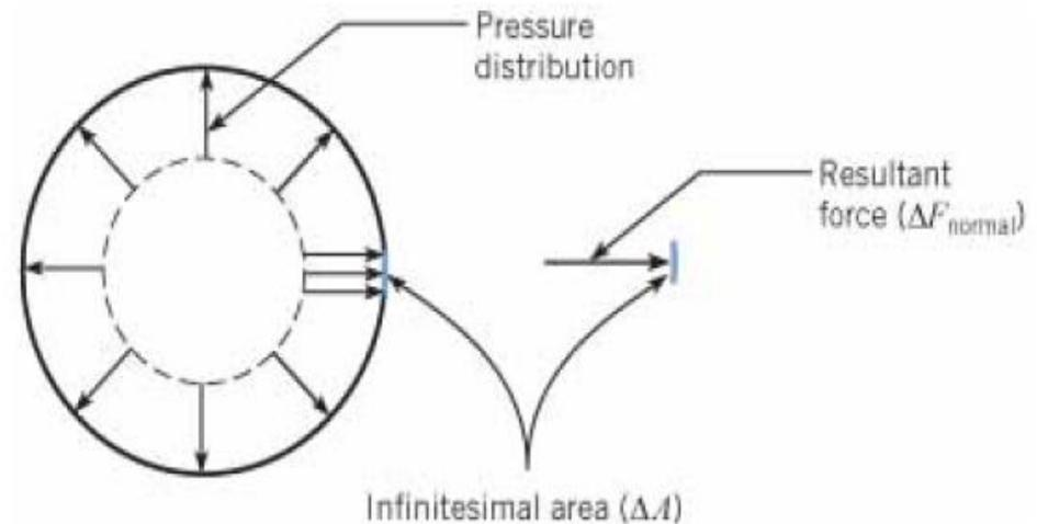
Figure 3.2 Pressure acting on the walls of a sphere.
