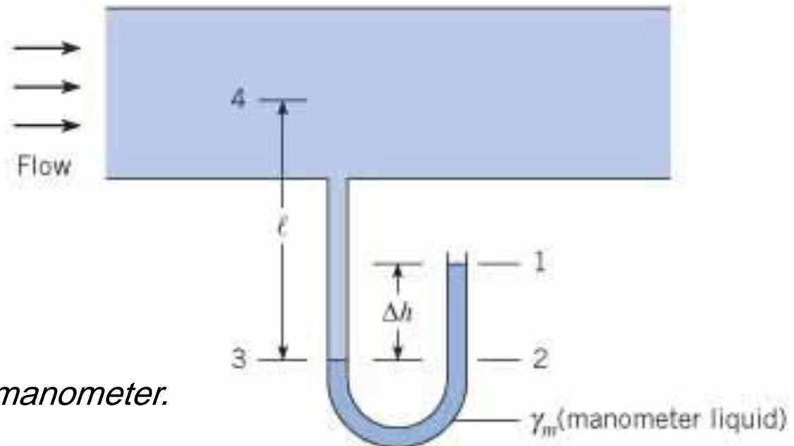
Figure 3.11 *U-tube manometer.*
