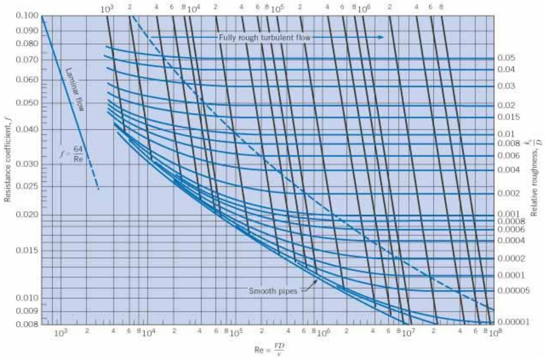
**Figure 10.13** Resistance coefficient  $f$  versus  $Re$ . Reprinted with minor variations. [After Moody 3.]
