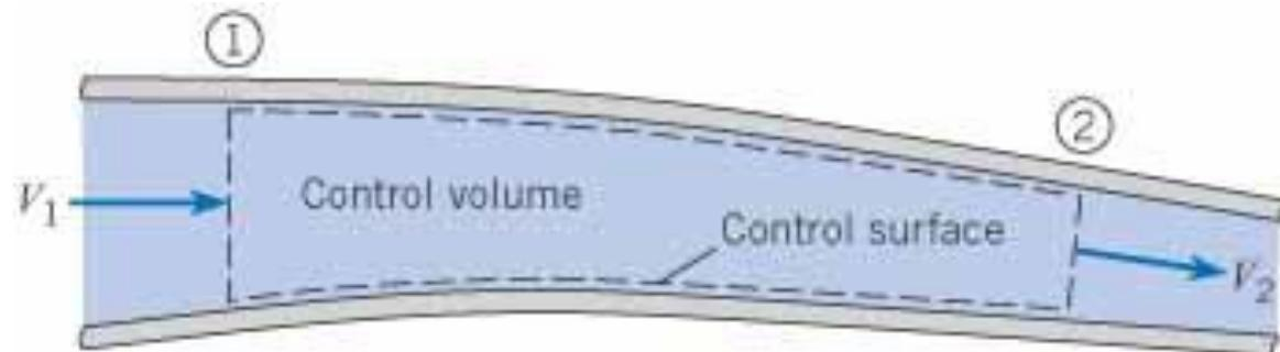
**Figure 5.7** *Flow through control volume in a duct.*
