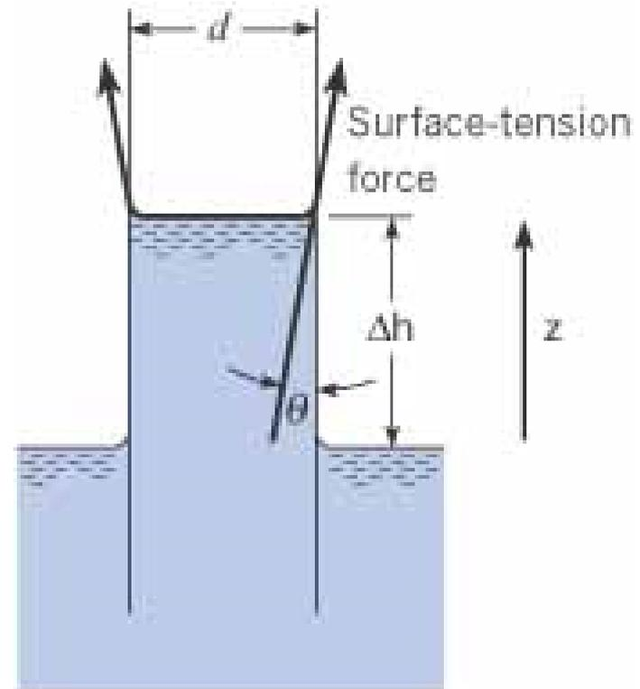
**Figure 2.7** *Capillary action in a small tube.*
