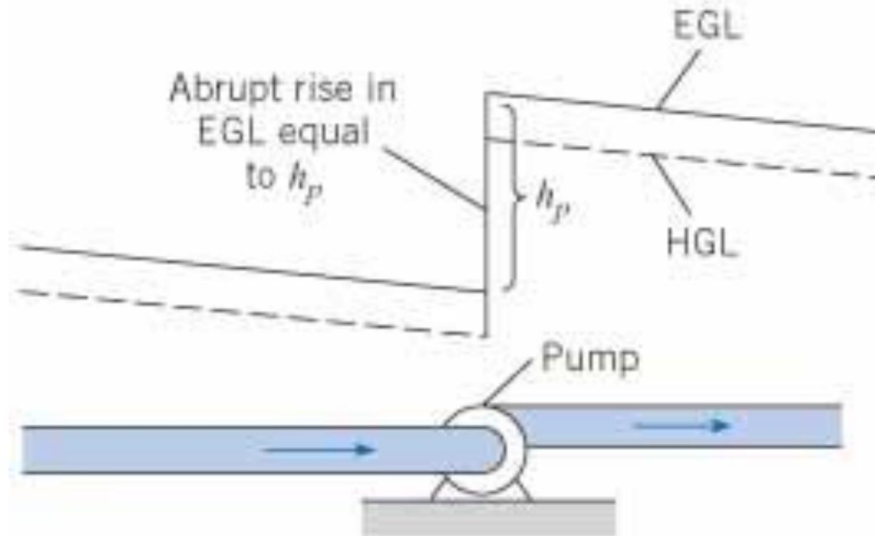
**Figure 7.8** *Rise in EGL and HGL due to Pump.*
