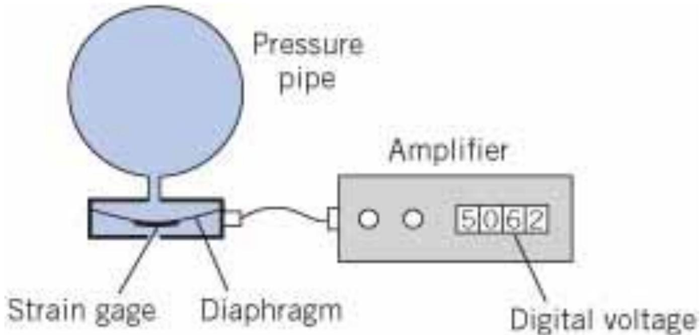
**Figure 3.13** *Schematic diagram of strain-gage pressure transducer.*
