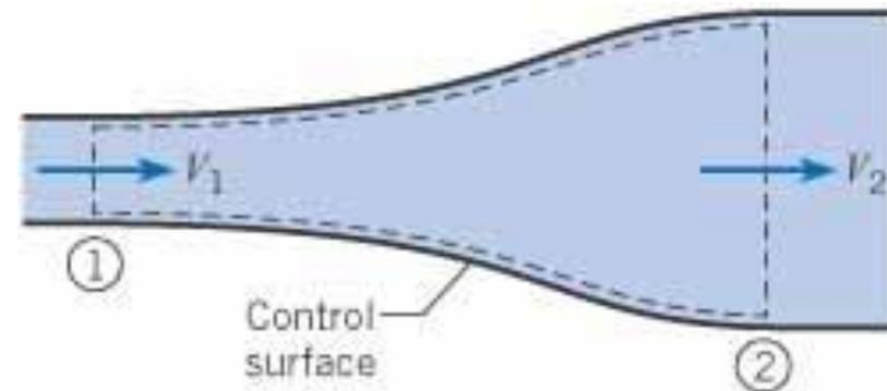
**Figure 5.10** *Flow through a pipe section.*
