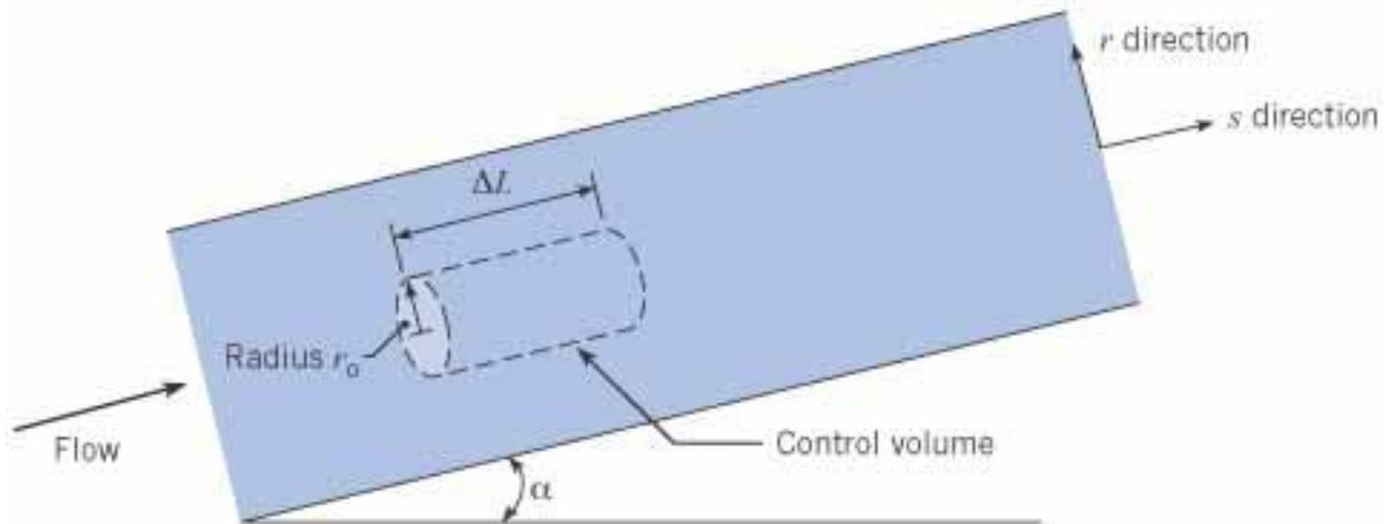
**Figure 10.7** Sketch for derivation of an equation for shear stress.
