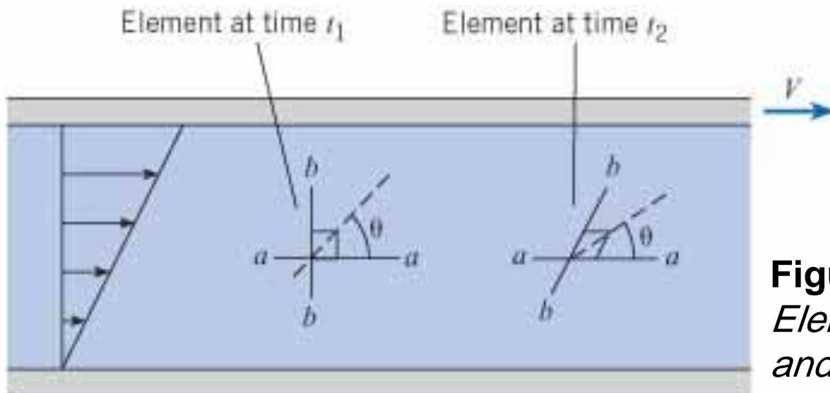
**Figure 4.16** *Rotation of a fluid Element in flow between a moving and stationary parallel plate.*
