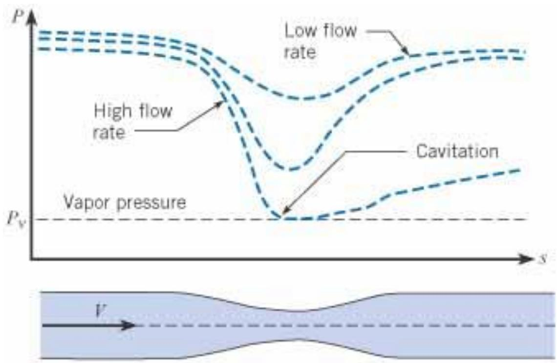
**Figure 5.11** *Flow through pipe restriction: variation of pressure for three different flow rates.*
