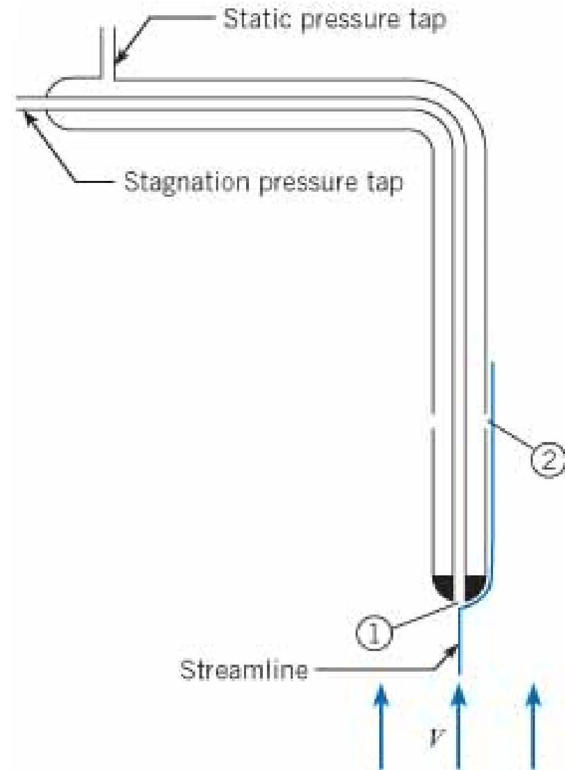
Figure 4.15 *Pitot-static tube.*
