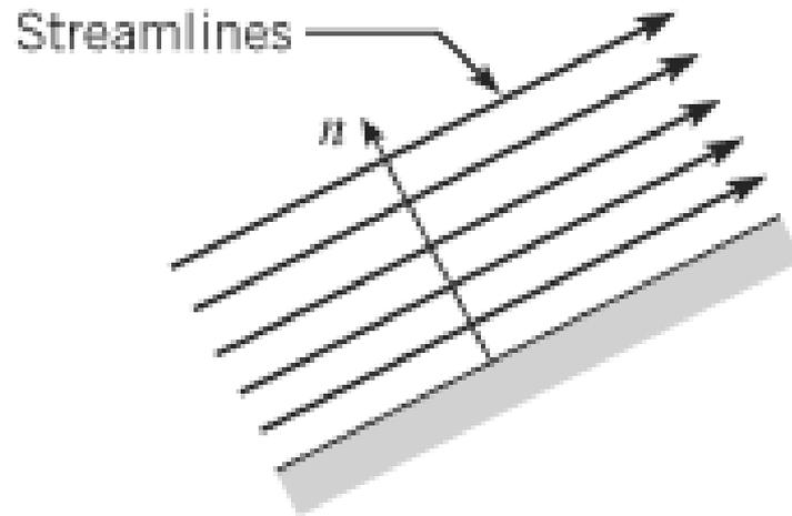
**Figure 4.12** *“Normal direction to parallel stream surface”*
