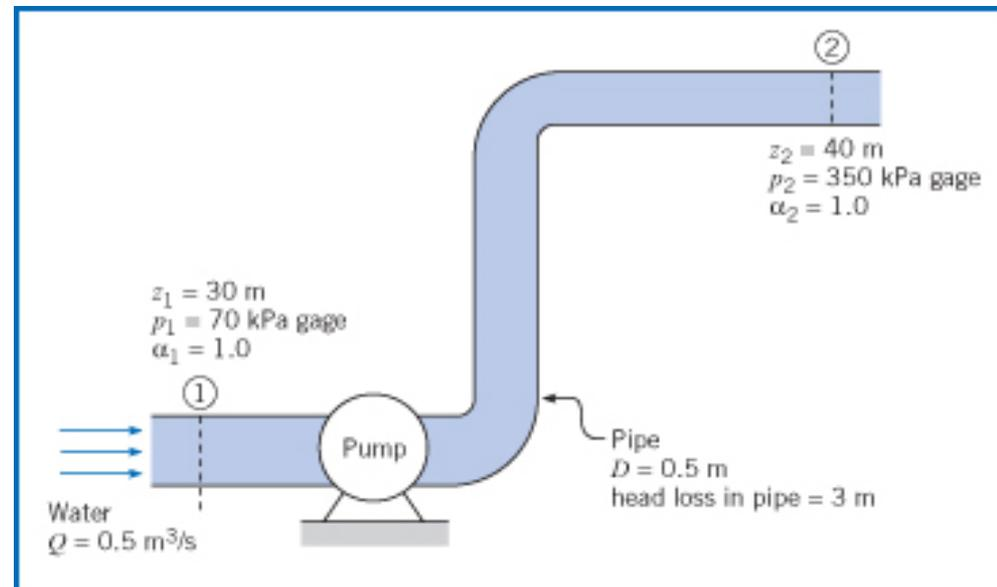
**Solution.** Apply the energy equation between sections 1 and 2,
