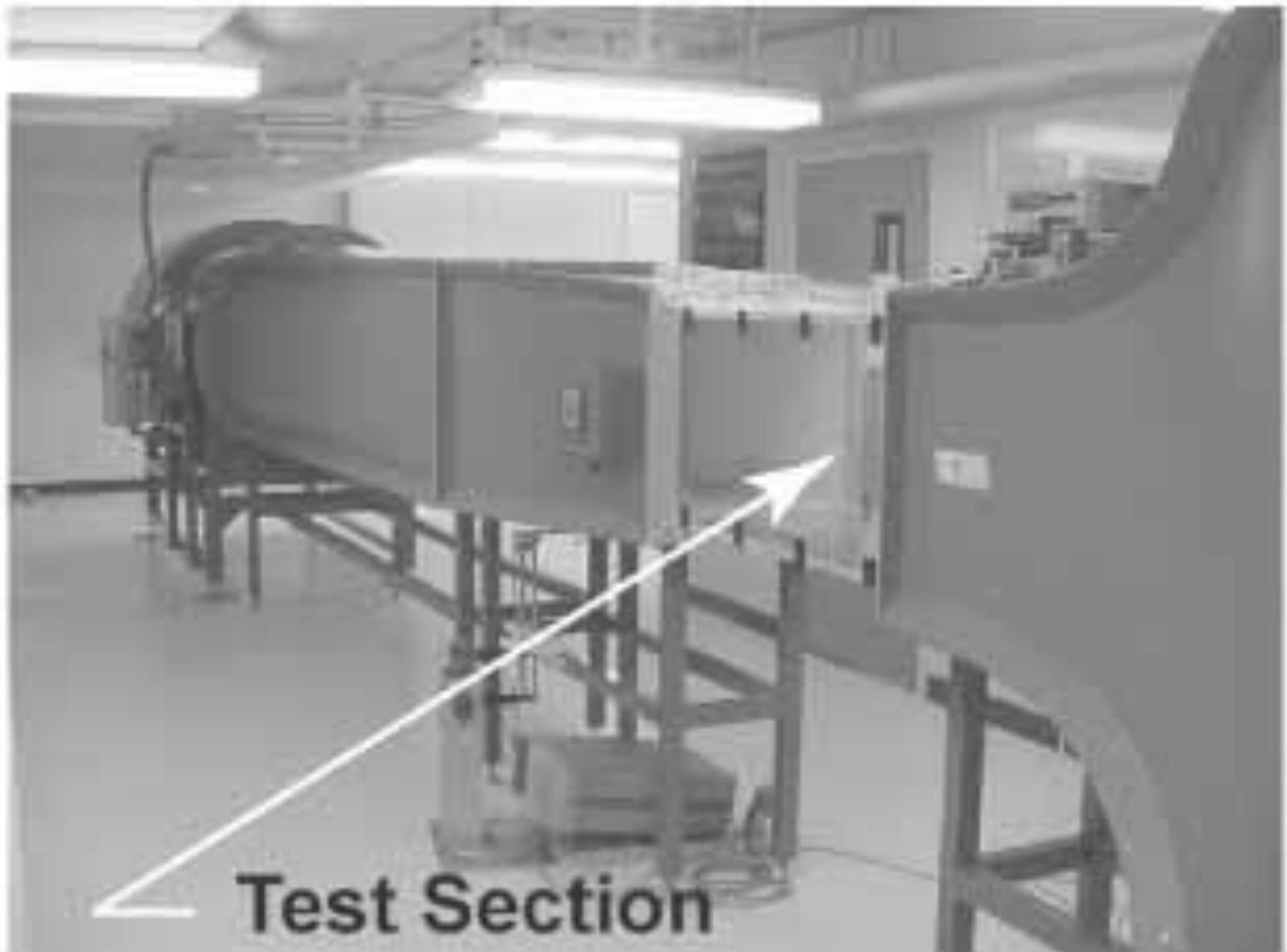
Wind tunnel used for testing flow over models.
