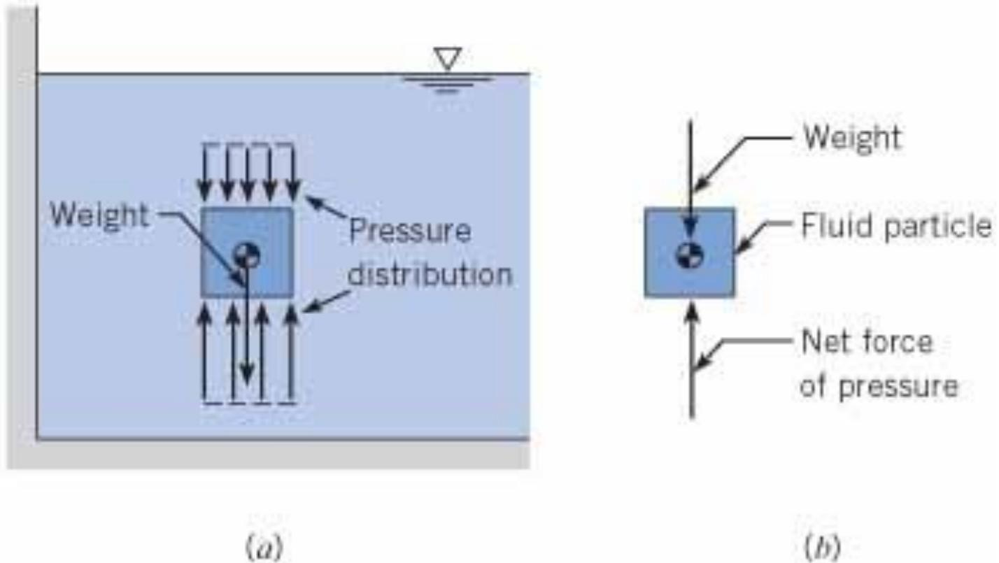
**Figure 3.1** *The hydrostatic condition.*
