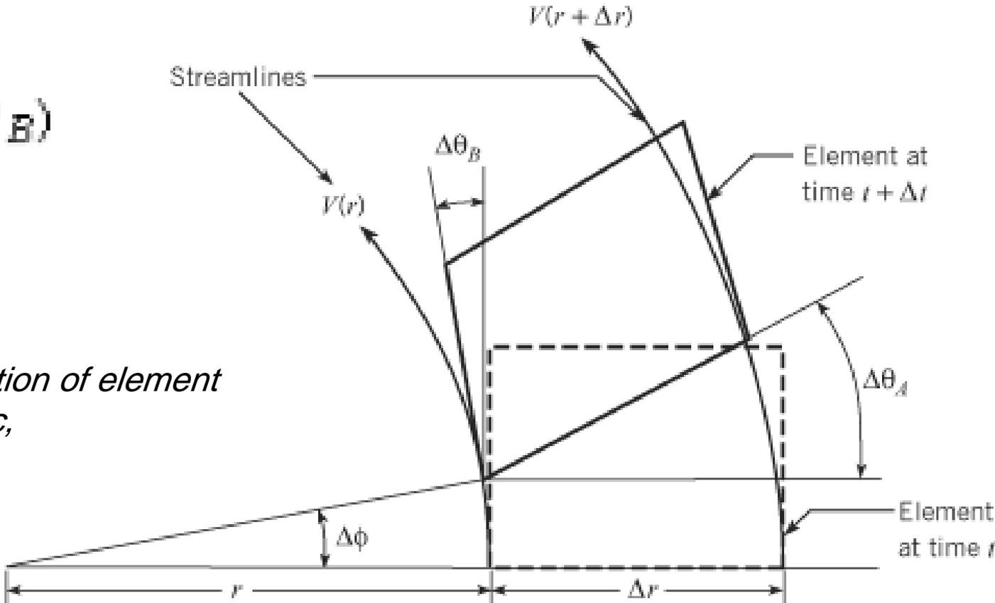
**Figure 4.19** Deformation of element in flow with concentric, circular streamlines.
