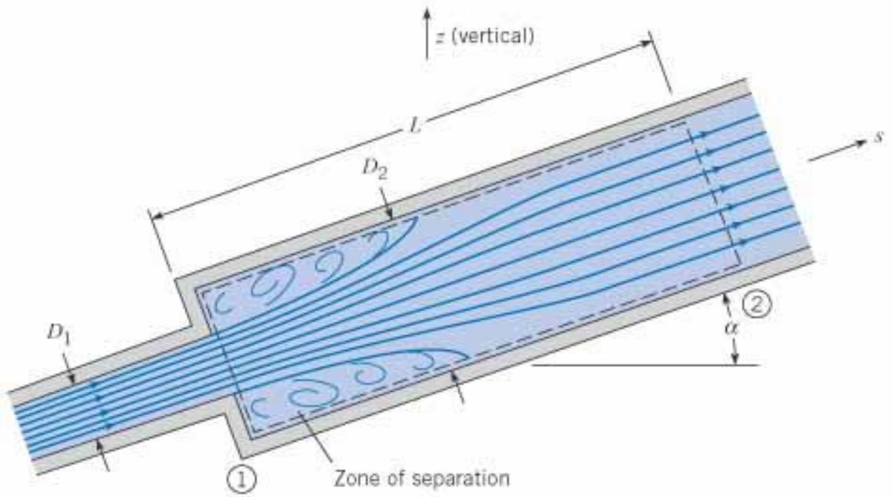
**Figure 7.6** *Flow through an abrupt expansion.*
