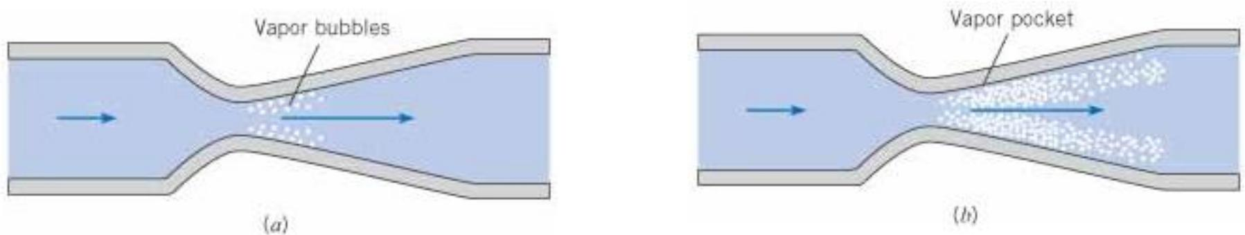
**Figure 5.12** *Formation of vapor bubbles in the process of cavitation.*
