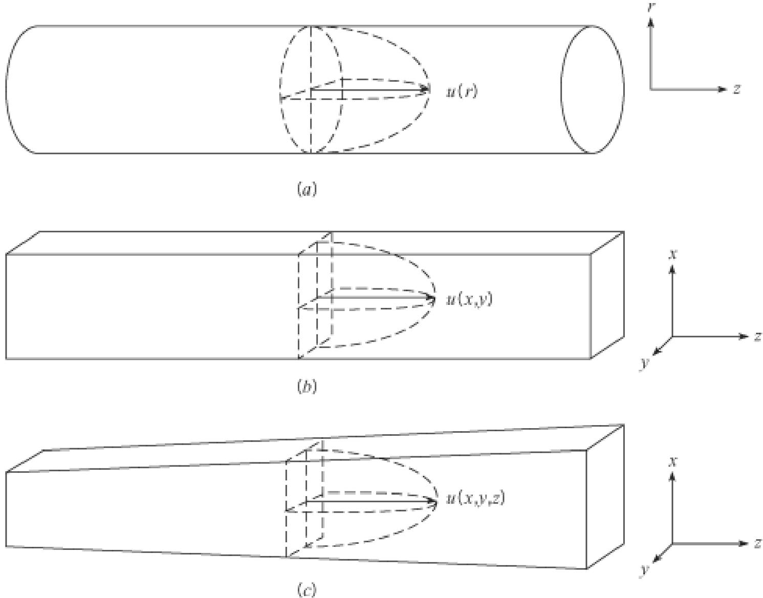
**Figure 4.8** *Flow dimensionality: (a) one-dimensional flow, (b) two-dimensional flow, and (c) Three-dimensional flow.*
