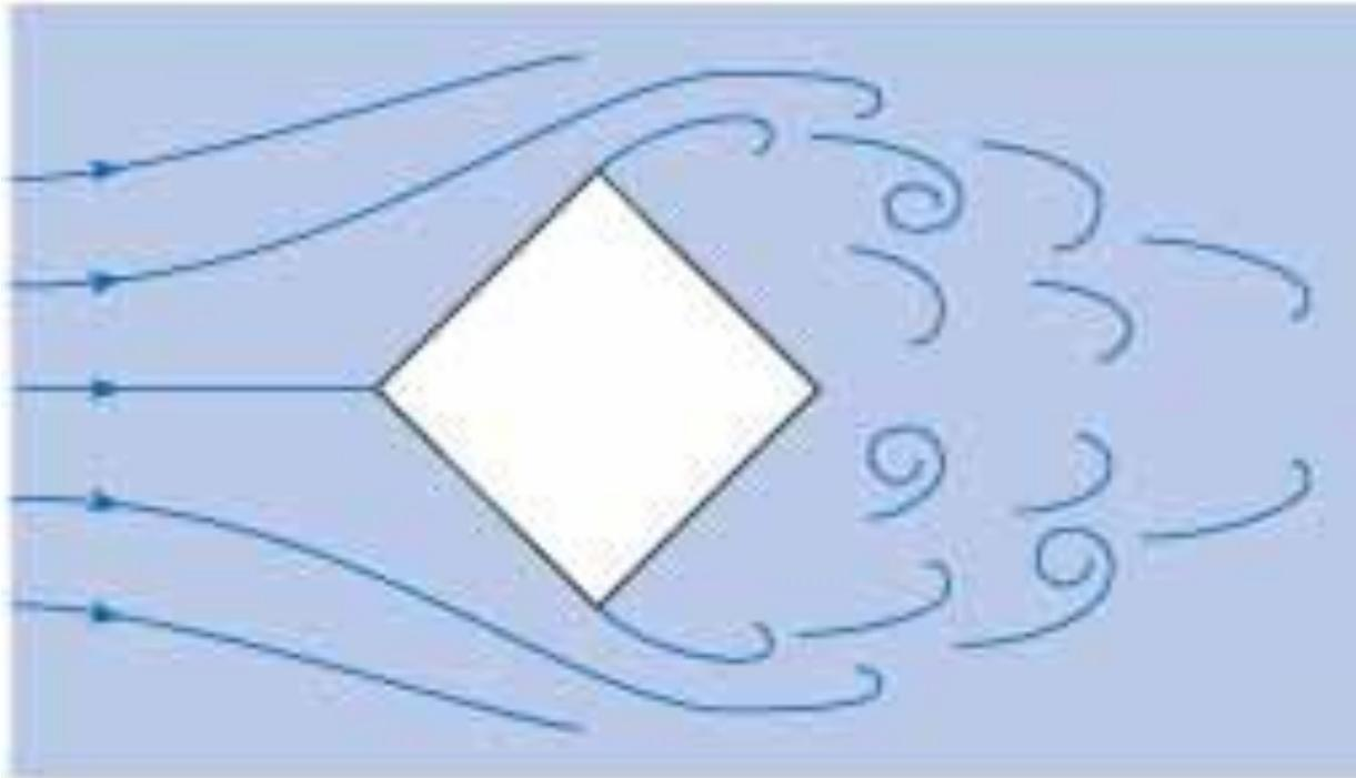
**Figure 4.27** *Flow pattern past a square rod illustrating separation at the edges.*
