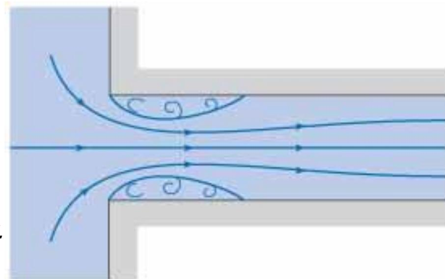
**Figure 10.15** *Flow at a sharp-edged inlet.*
