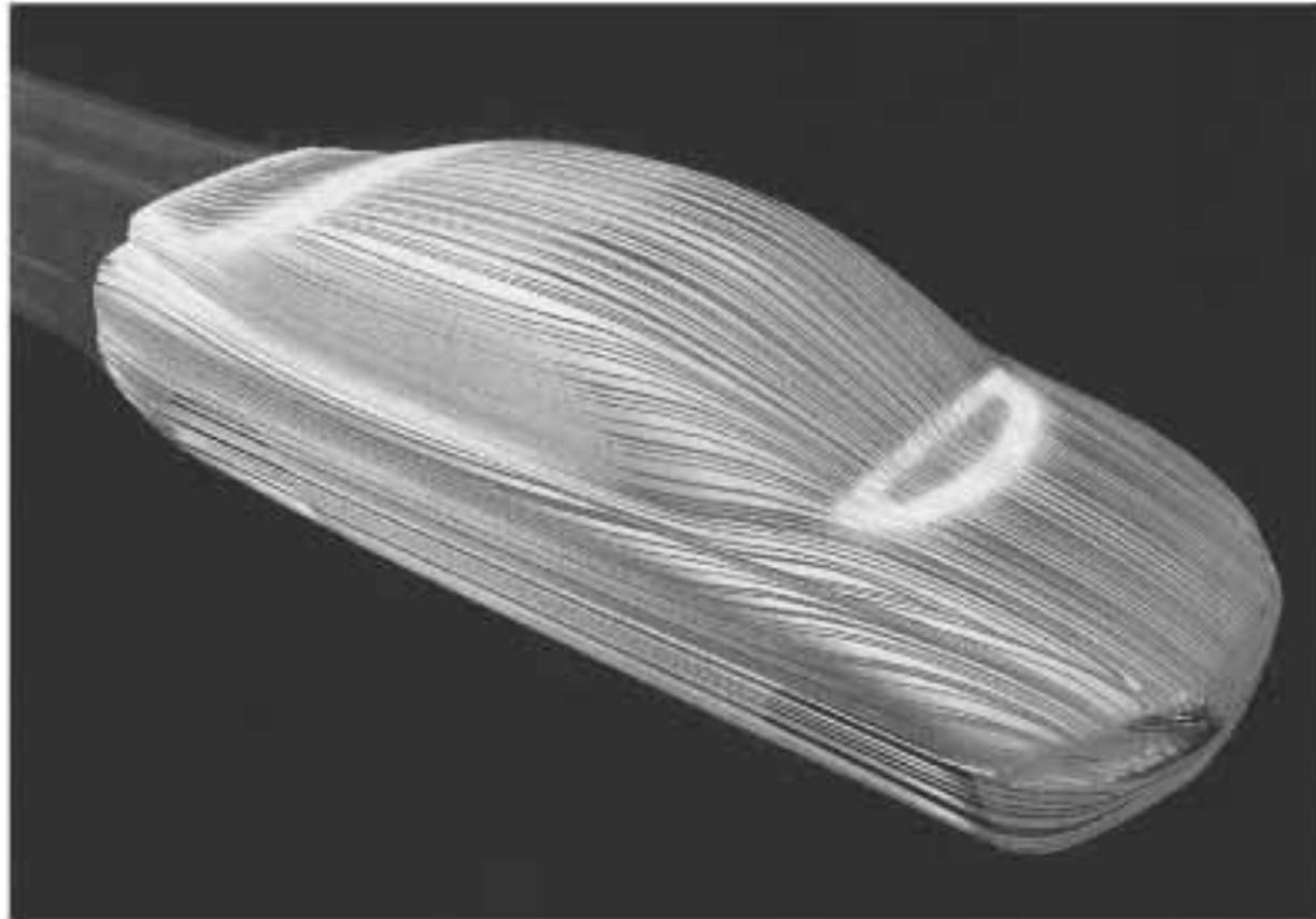
**Figure 4.2** *Predicted streamline pattern over the Volvo ECC prototype.*
