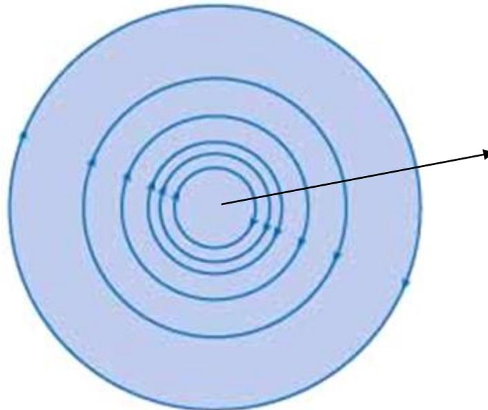
Apply Euler's equation in the direction normal to the streamlines and outward from the center of rotation. In this case the fluid elements rotate as a rigid body, so the direction  $l$  in Euler's equation is replaced by  $r$  giving
