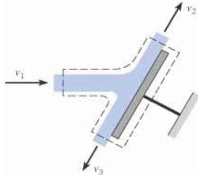
**Figure 6.4** *Fluid jet striking a flat vane.*
