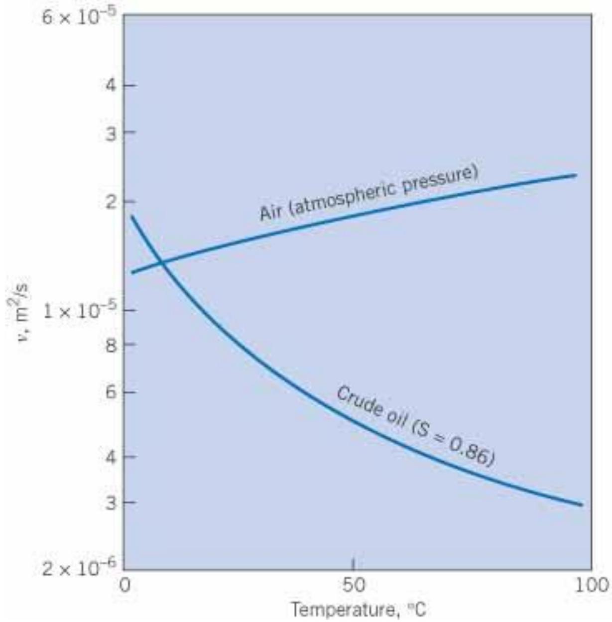
**Figure 2.3** *Kinematic viscosity for air and crude oil.*
