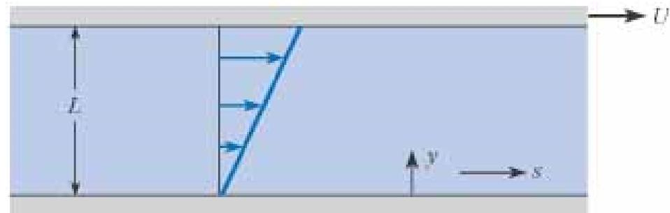
Figure 9.2 Flow generated by a moving plate (Couette flow).
