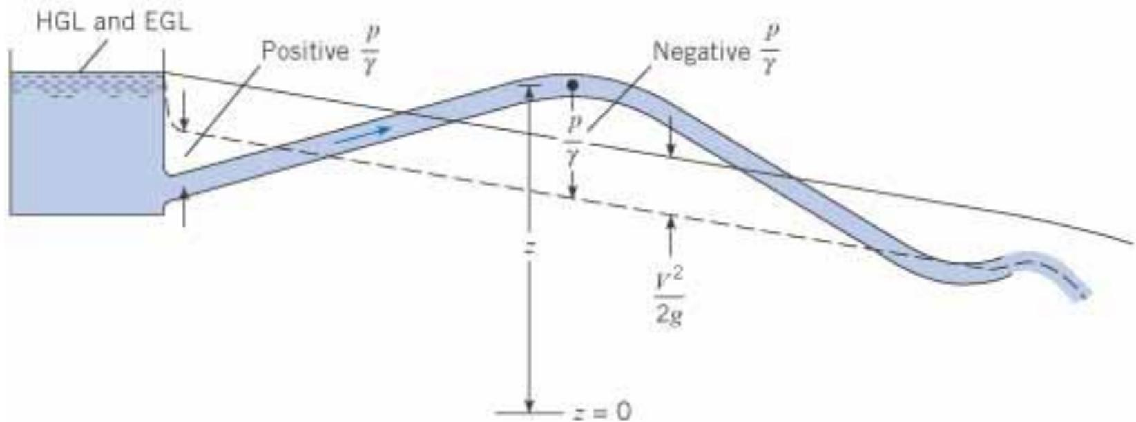
**Figure 7.12** *Subatmospheric pressure when pipe is above HGL.*
