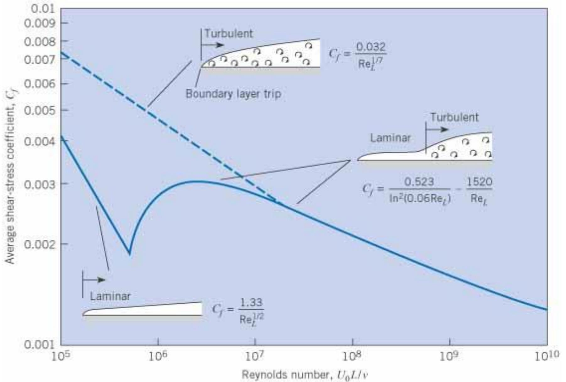
**Figure 9.12** Average shear-stress coefficients.
