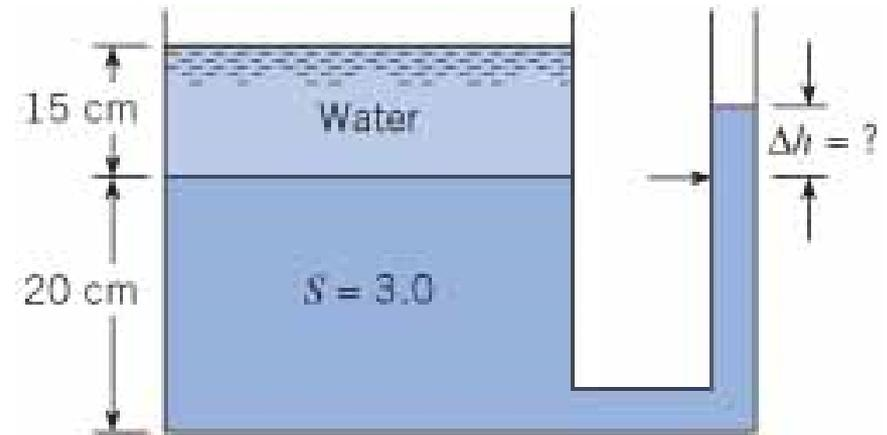
**3.30** Is the gage pressure at the center of the pipe (a) negative, (b) zero, or (c) positive? Neglect surface tension effects and state your rationale. Note, solve in SI units.
