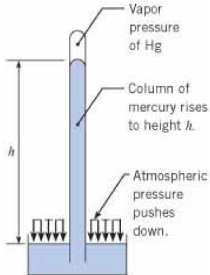
**Figure 3.8** *A mercury barometer.*
