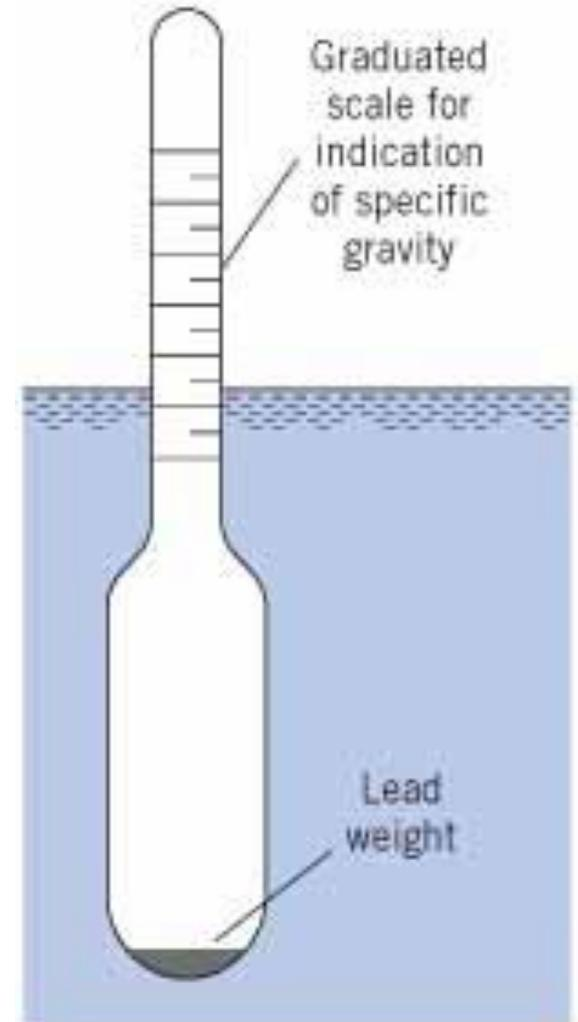
**Figure 3.22** *Hydrometer*
