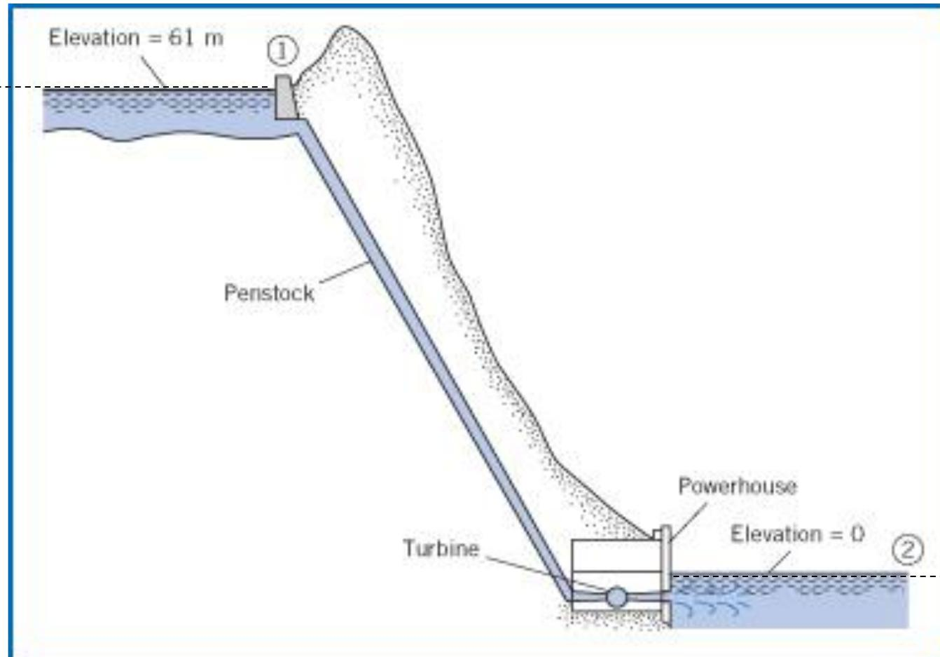
**Solution.** Apply the energy equation between sections 1 and 2,
