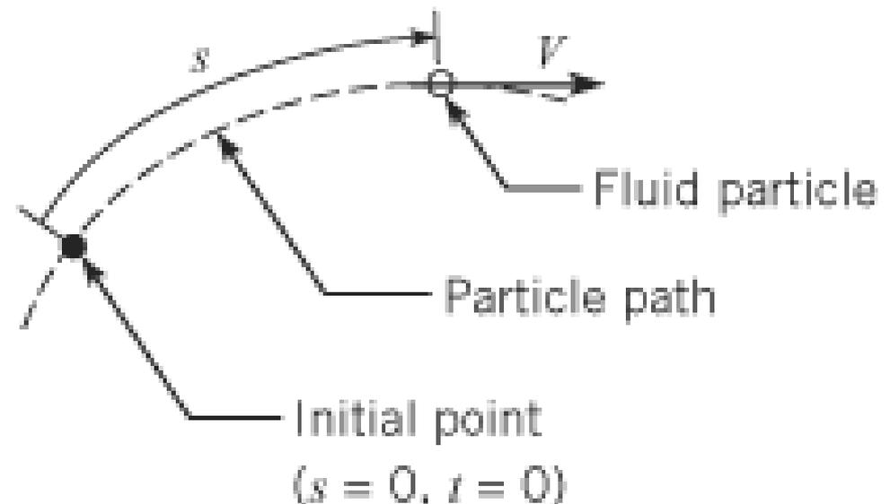
**Figure 4.3** *Fluid particle moving along a pathline.*
