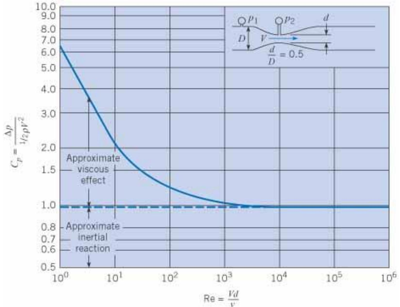
**Figure 8.6**  $C_p$  for a venturi meter as a function of the Reynolds number
