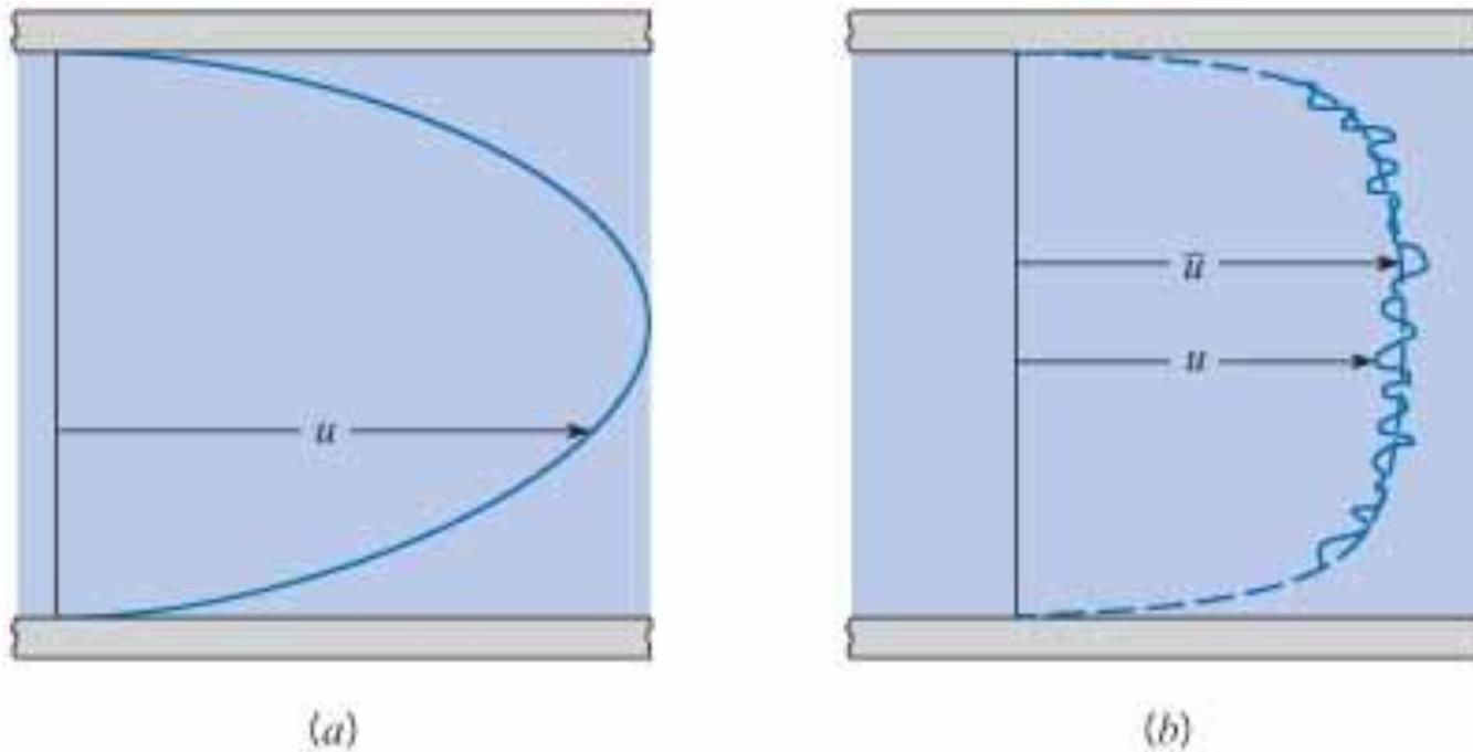
**Figure 4.7** *Laminar and turbulent flow in a straight pipe.*
