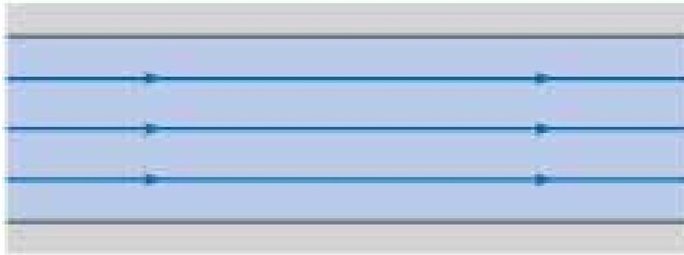
**Figure 4.4** *Uniform flow in a pipe.*
