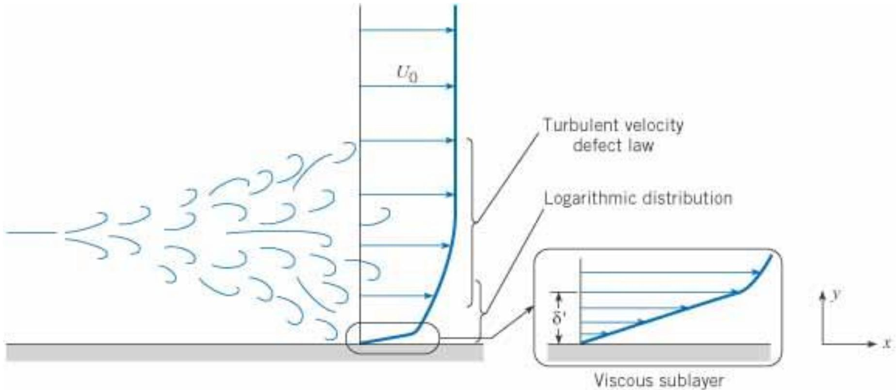
**Figure 9.6** *Sketch of zones in turbulent boundary layer.*
