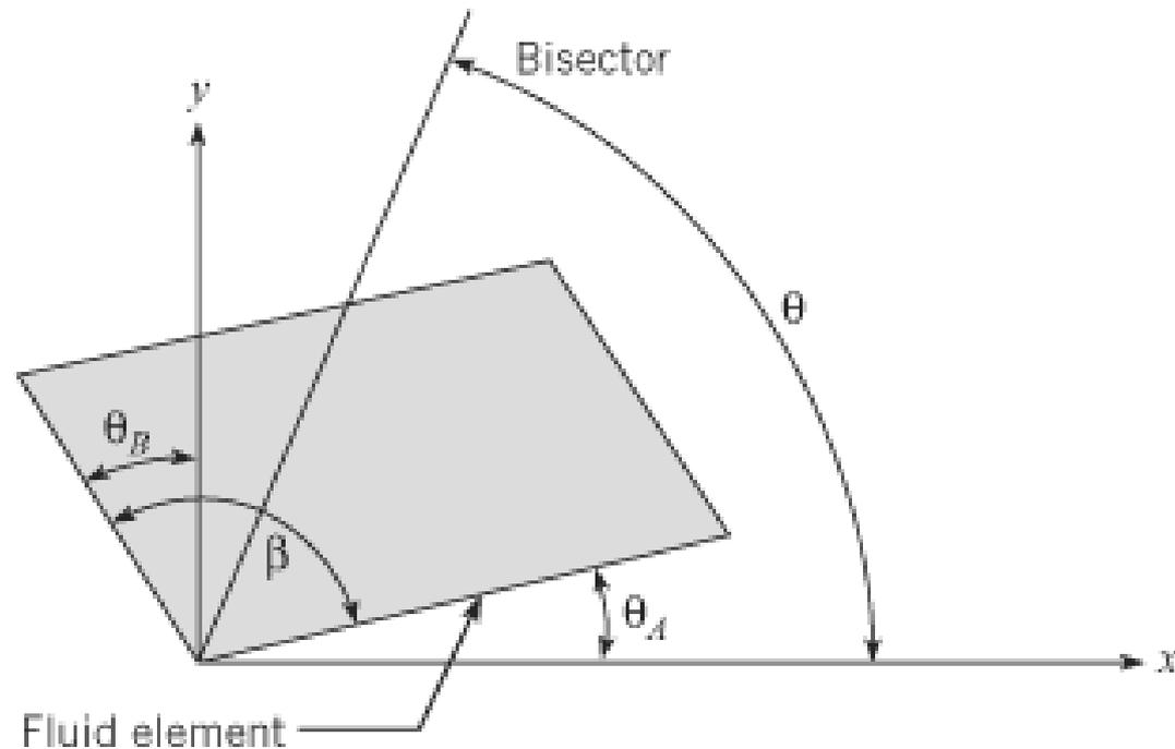
**Figure 4.17** *Orientation of rotated fluid element.*
