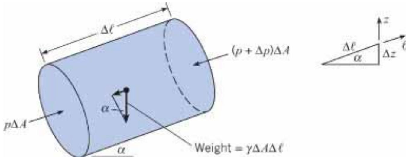
**Figure 3.5** *Variation in pressure with elevation.*
