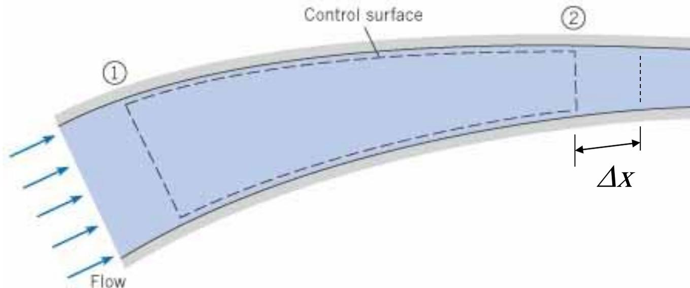
**Figure 7.3** Sketch for deriving flow work.
