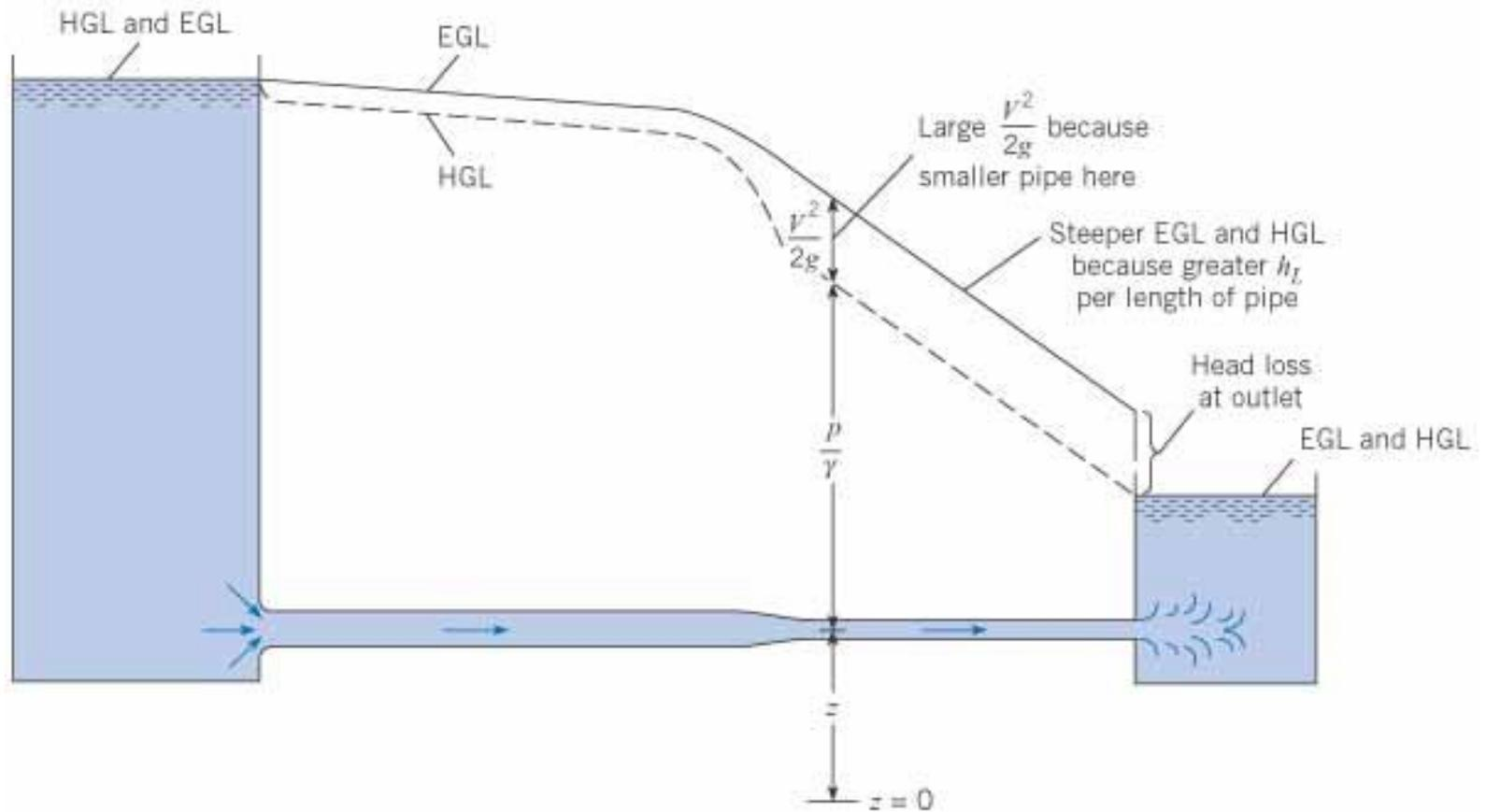
**Figure 7.11** *Change in EGL and HGL due to change in diameter of pipe.*
