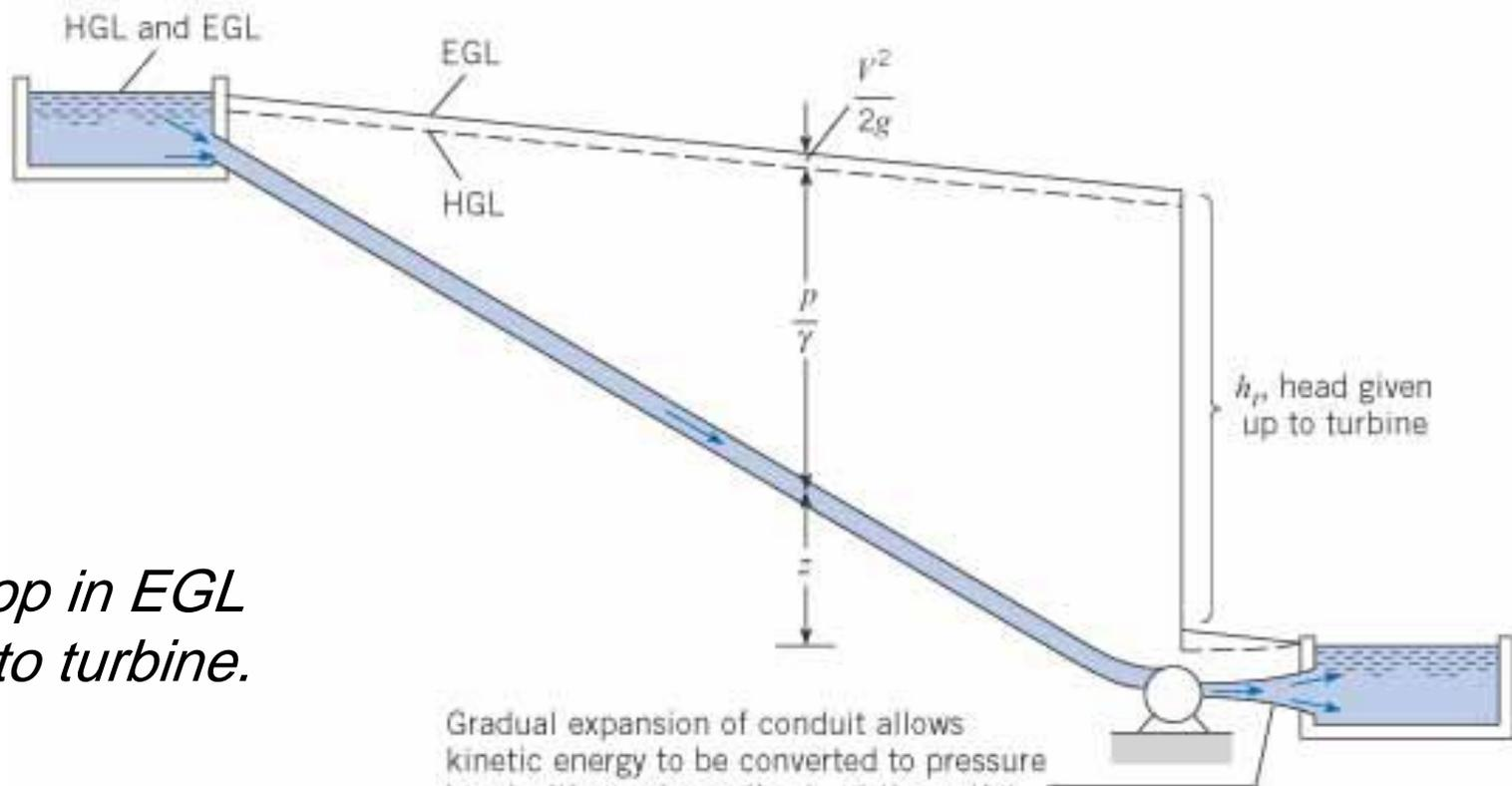
Gradual expansion of conduit allows kinetic energy to be converted to pressure head with much smaller  $h_t$  at the outlet; hence the HGL approaches the EGL.
