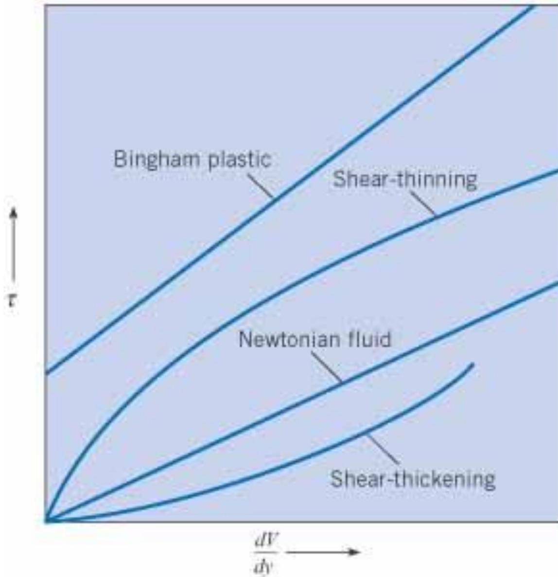
**Figure 2.6** *Shear stress relations for different types of fluids.*
