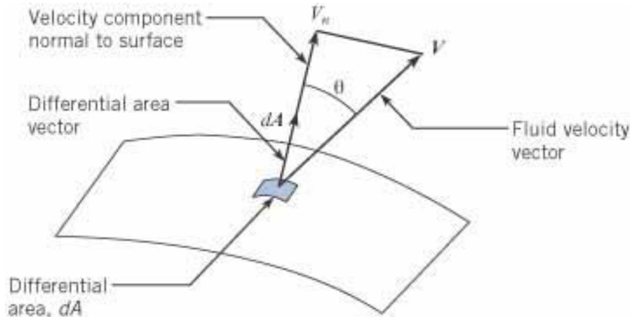
**Figure 5.5** *Velocity vector oriented at angle  $\theta$  with respect to normal.*
