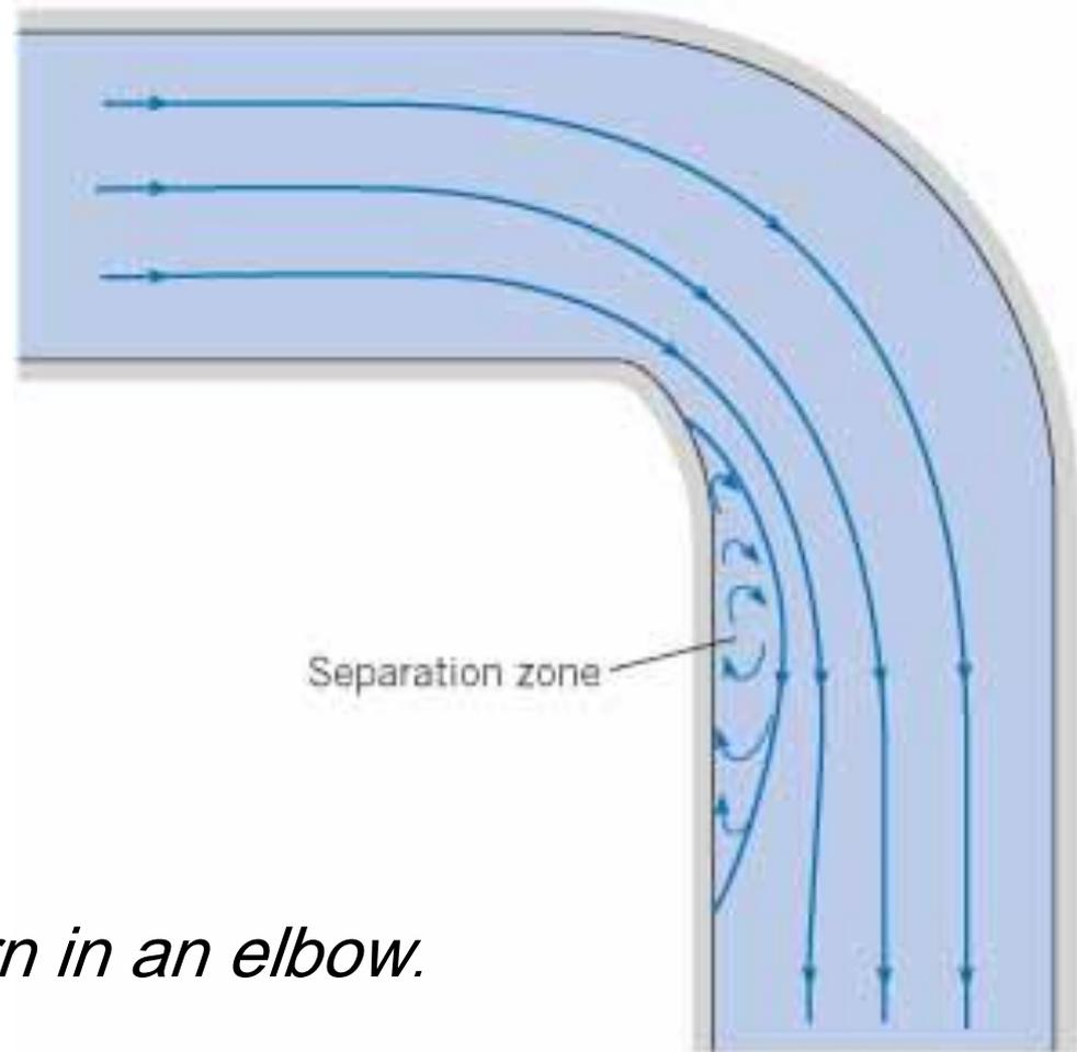
**Figure 10.16** *Flow pattern in an elbow.*
