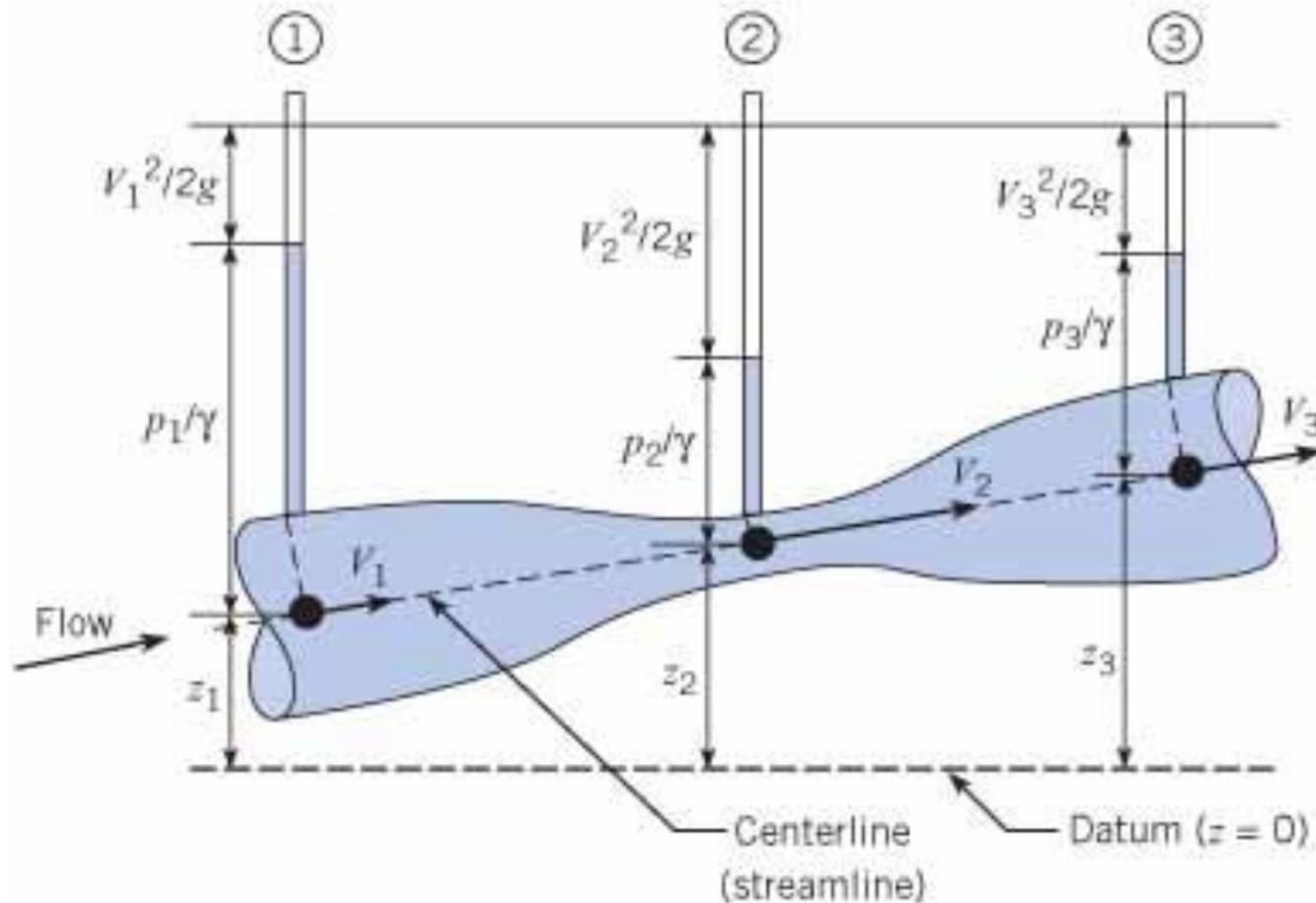
**Figure 4.13** Piezometric and velocity head variation for flow through a venturi section.
