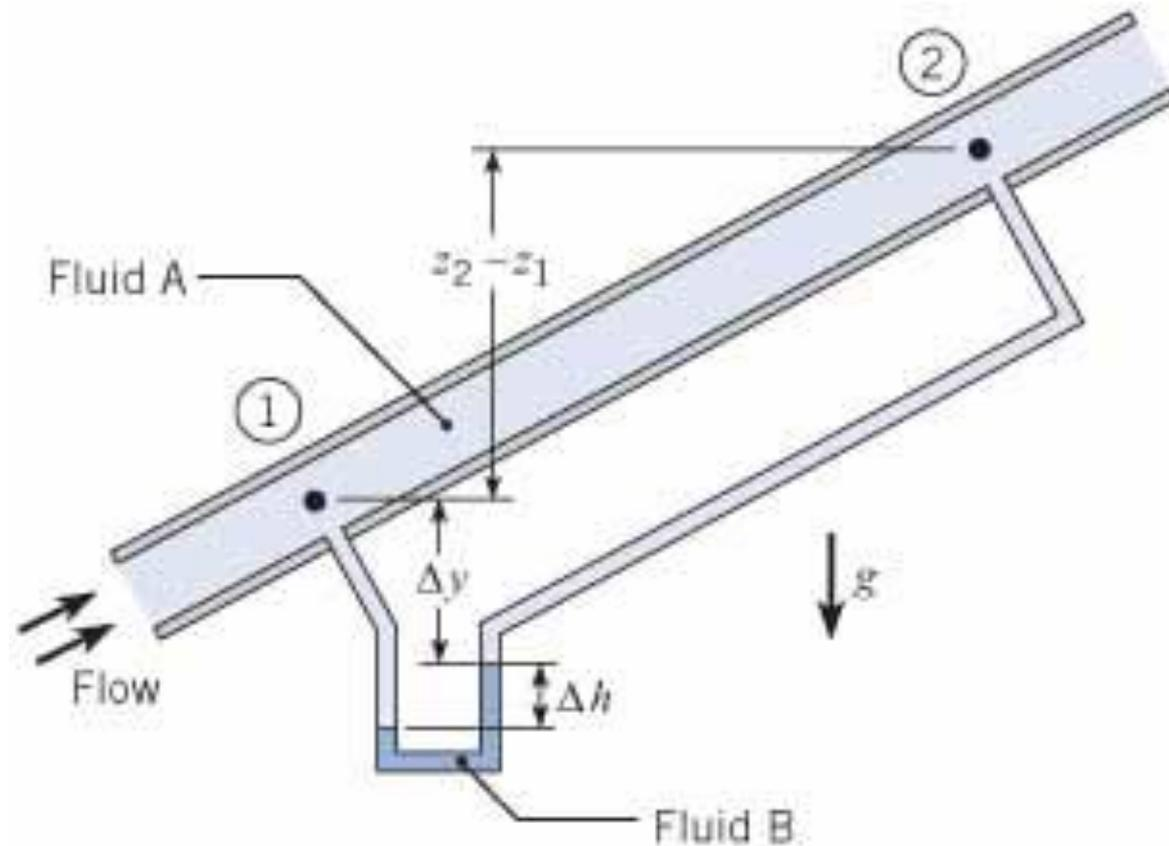
**Figure 3.12** Apparatus for determining change in piezometric head corresponding to flow in a pipe.
