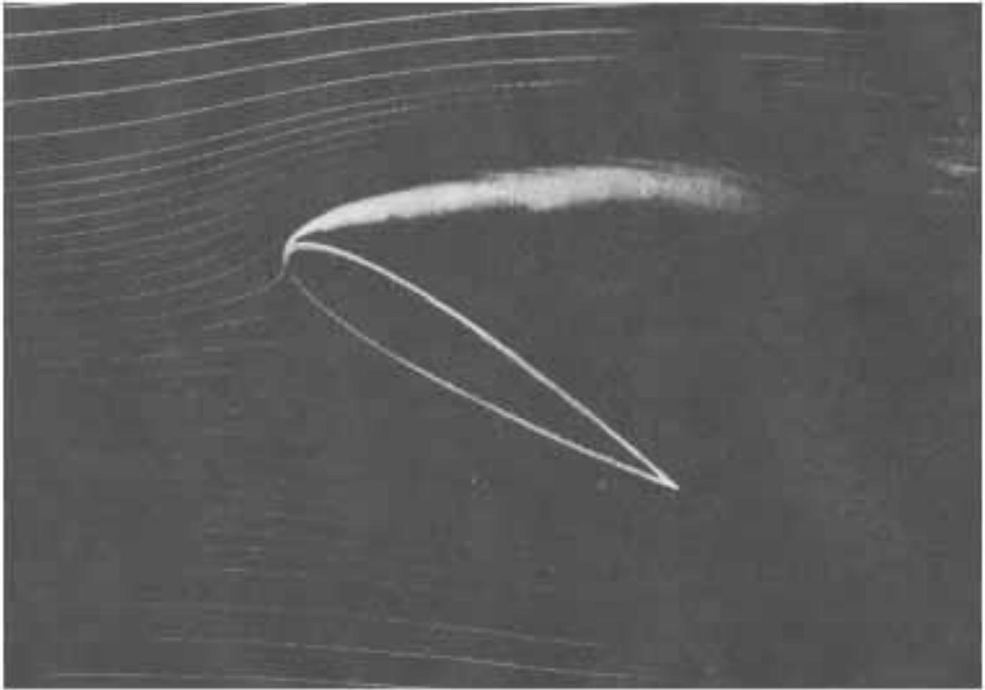
**Figure 4.26** *Smoke traces showing separation on an airfoil section at a large angle of attack. (Courtesy of Education Development Center, Inc. Newton, MA)*
