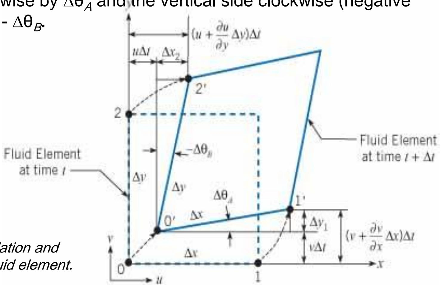
**Figure 4.18** Translation and deformation of a fluid element.
