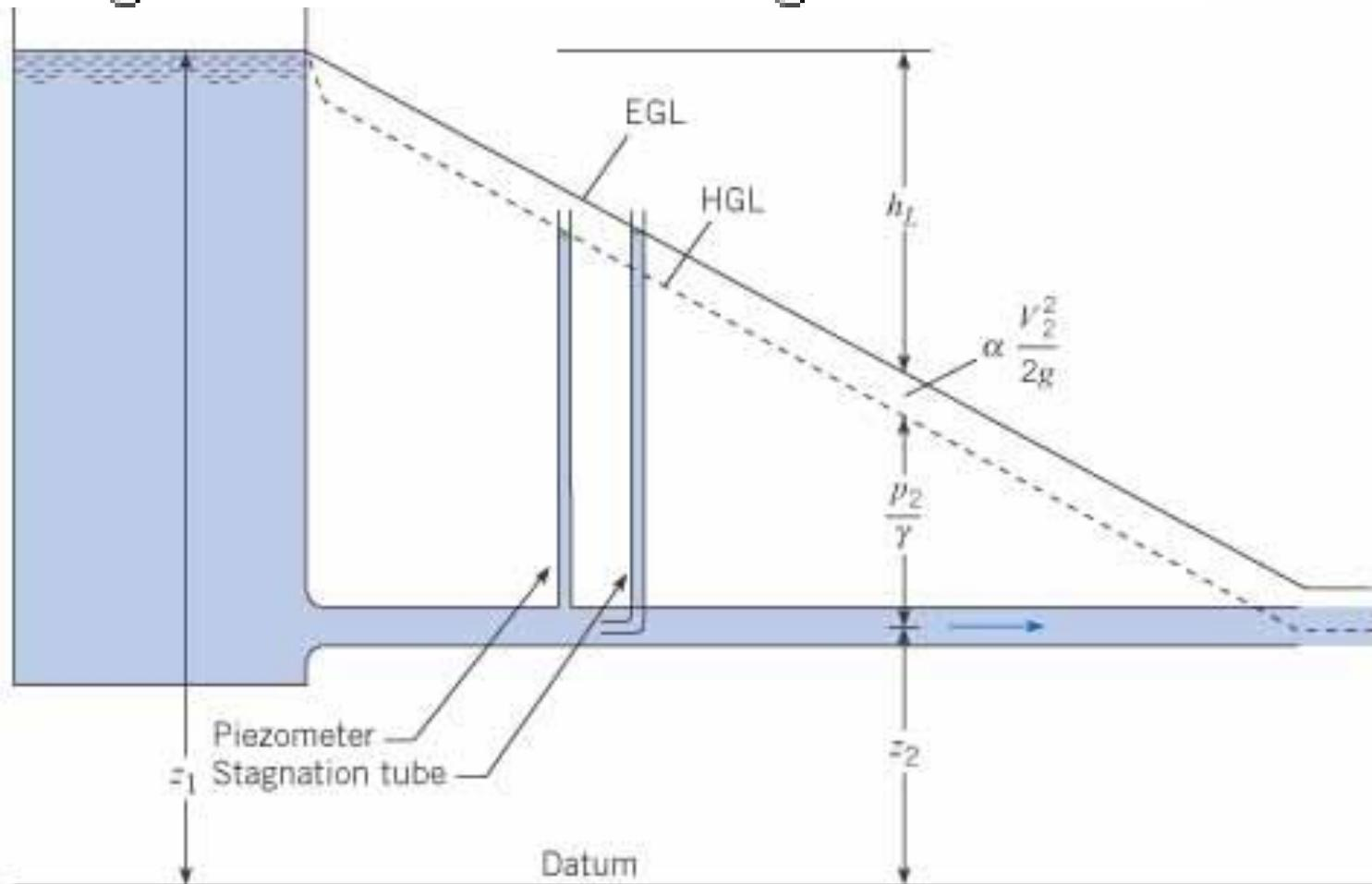
**Figure 7.7** *EGL and HGL in a straight pipe.*
