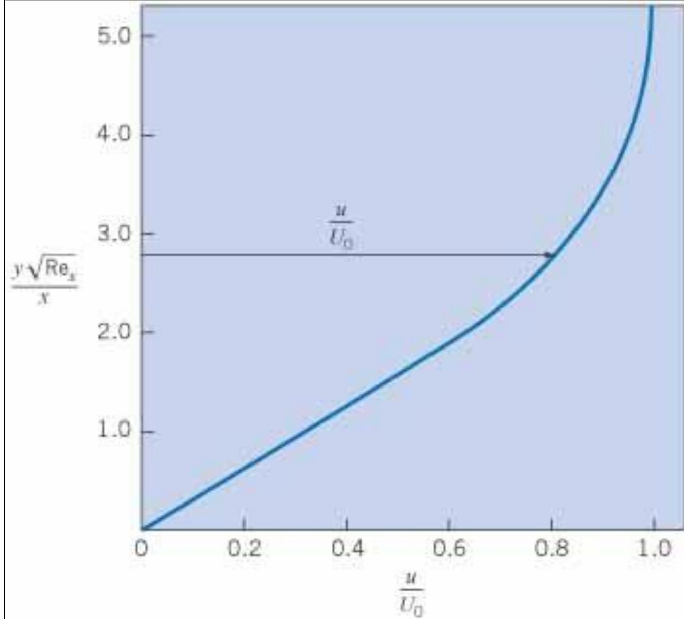
**Figure 9.5** *Velocity distribution in laminar boundary layer.*
