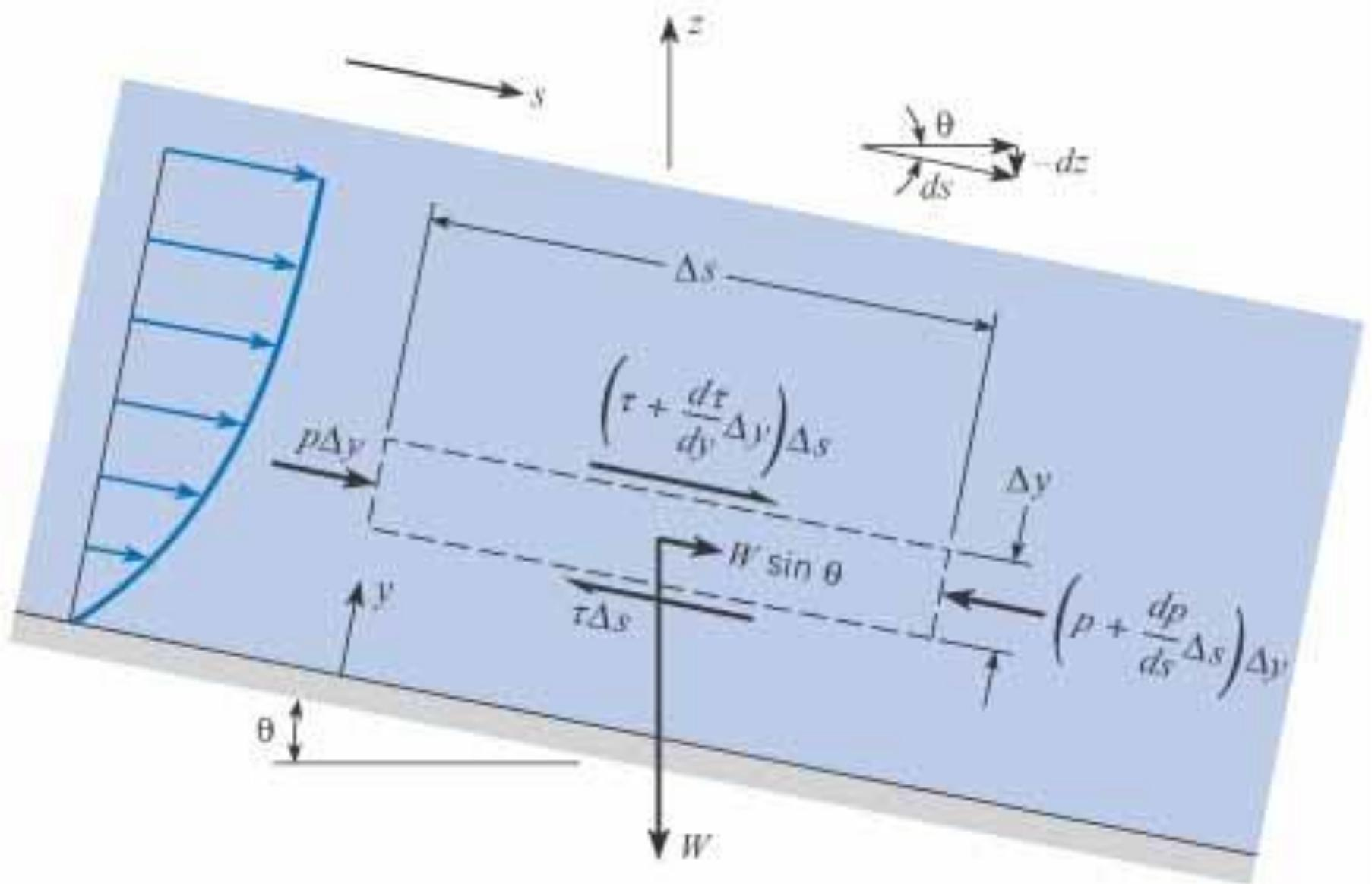
**Figure 9.1** *Control volume for analysis of uniform flow with parallel streamlines.*
