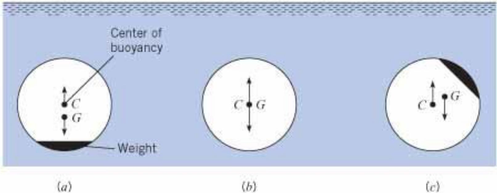
**Figure 3.23** *Conditions of stability for immersed bodies.*
