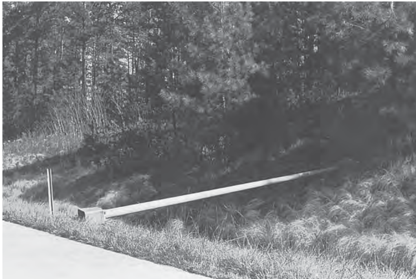
FIGURE 7.79 Failure of luminaire support without impact.
