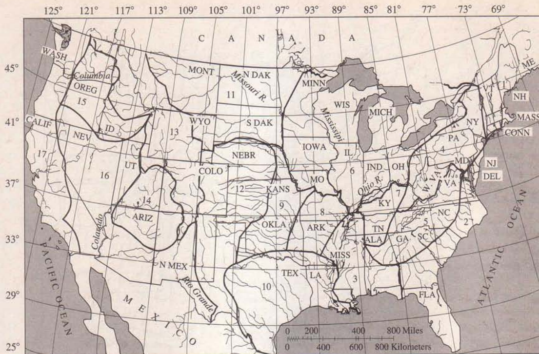
Figure 16.29 Map of the conterminous United States showing Crippen and Bue flood region boundaries. (Source: After U.S.G.S. Water Supply Paper 1887).
