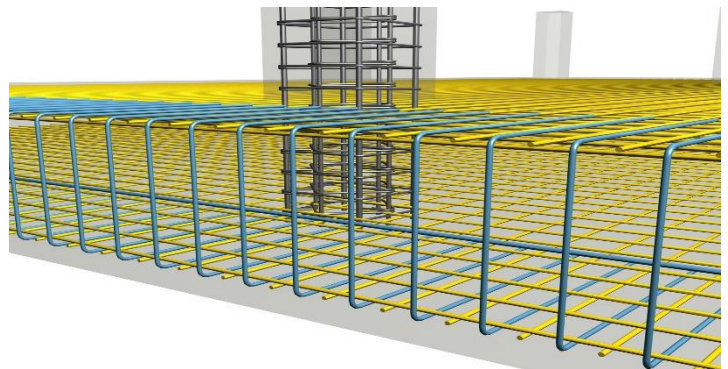
Figure 7.5: bent the steel at the end of foundation
