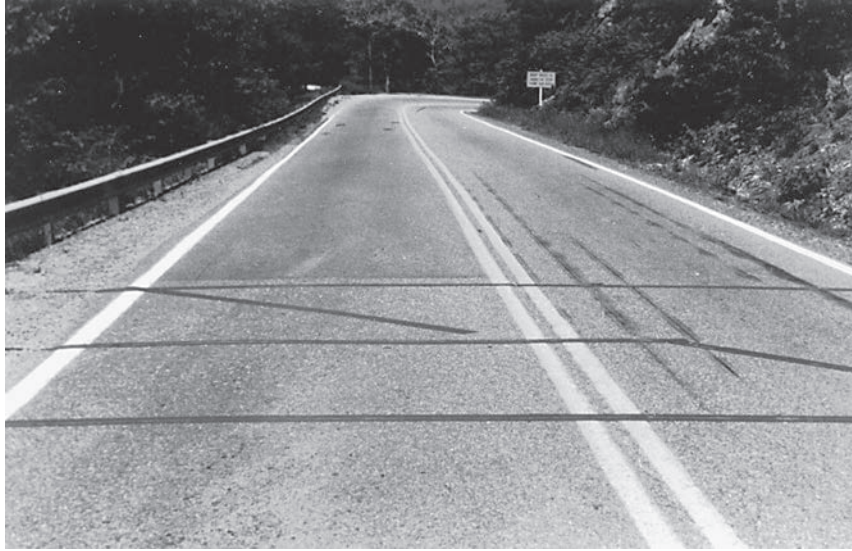
Figure 4.3 An Example of a Sensor Setup of a Surface Detector Using Pneumatic Road Tubes
