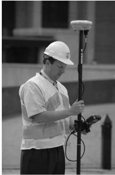
Figure 14.5 "Trimble 5800" Setup for RTK (Real-Time Kinematic) Data Collection
