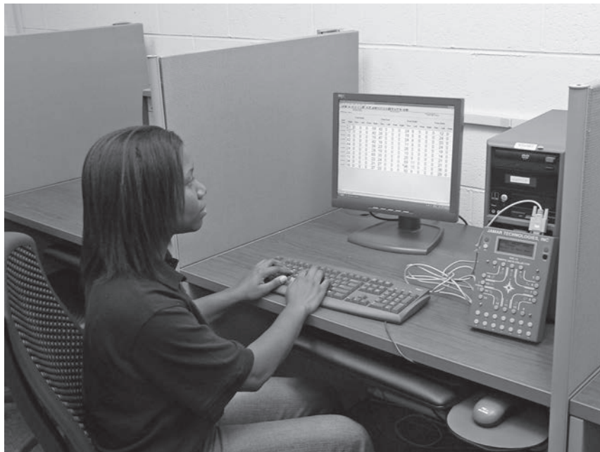
Figure 4.5 Jamar Technologies Traffic Data Collector TDC-12 Hooked to a Computer
