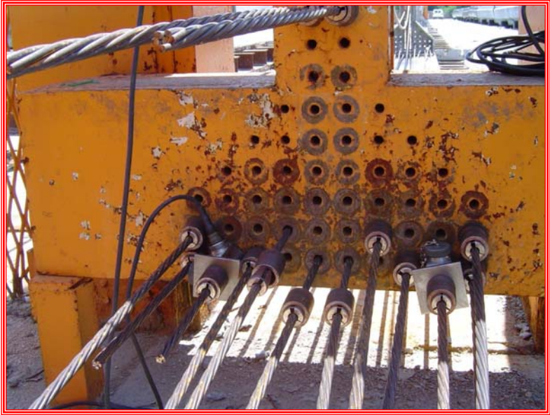
View of the lower flange tendons with load cells installed (Dead End)
