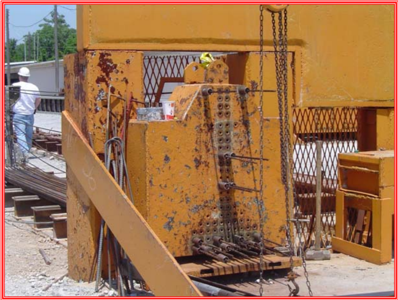
View of all tendons with load cells installed (Dead End)
