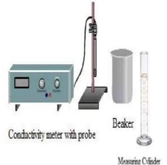
Figure 7.1: Apparatus of Conductivity experiment
