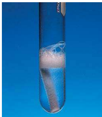
Figure 4.6 A piece of blackboard chalk, which is mostly \text{CaCO}_3 , reacts with hydrochloric acid.
