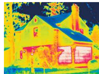
This infrared photo shows where energy (heat) leaks through the house. The more red the color, the more energy is lost to the outside.
