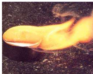
White phosphorus burns in air to form \text{P}_4\text{O}_{10} .
