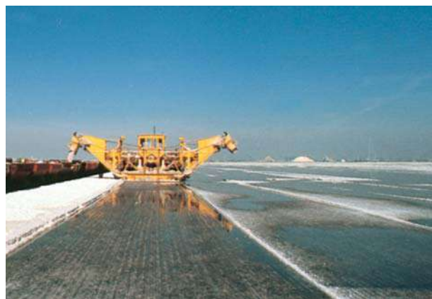
Solar evaporation process for obtaining sodium chloride.
