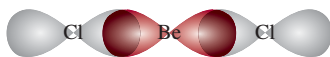
Figure 10.11 The linear geometry of \text{BeCl}_2 can be explained by assuming that Be is sp -hybridized. The two sp hybrid orbitals overlap with the two chlorine 3p orbitals to form two covalent bonds.
