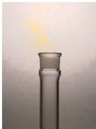
\text{N}_2\text{O}_5 decomposes to give \text{NO}_2 (brown color).
