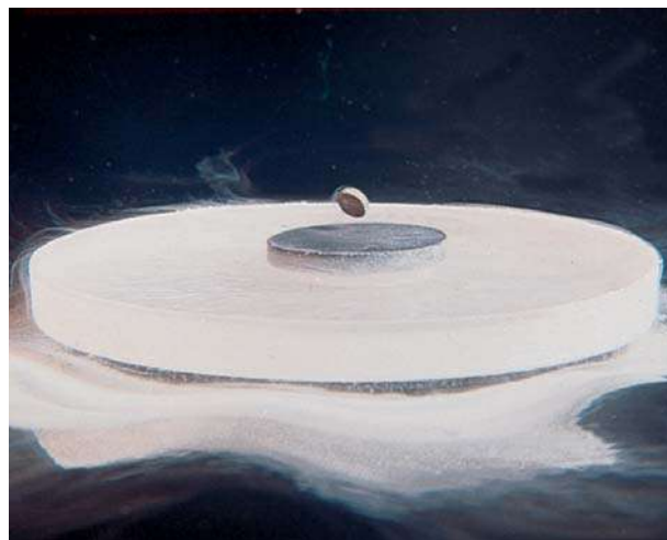
The levitation of a magnet above a high-temperature superconductor immersed in liquid nitrogen.
