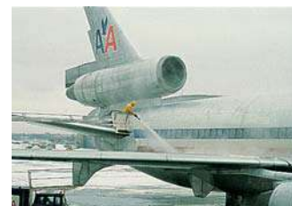
De-icing of airplanes is based on freezing-point depression.
