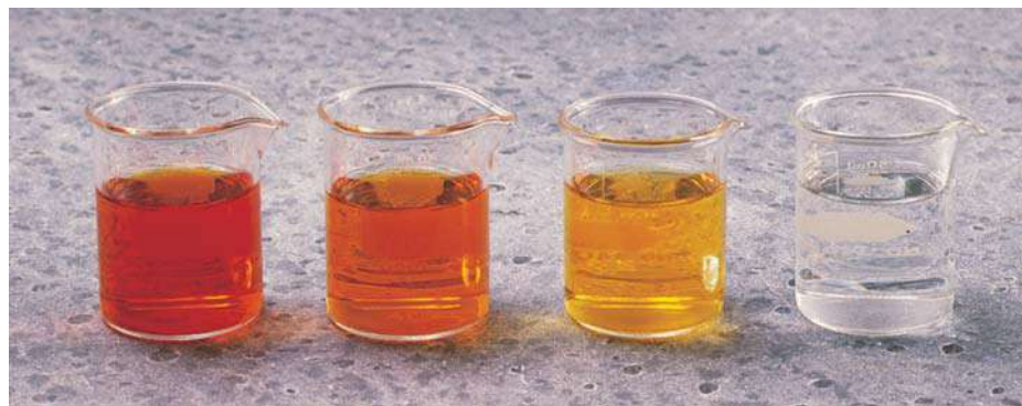
Figure 13.3 From left to right: The decrease in bromine concentration as time elapses shows up as a loss of color (from left to right).
