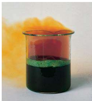
Figure 21.7 The production of \text{NO}_2 gas when copper reacts with concentrated nitric acid.
