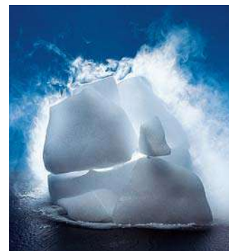
Figure 11.42 Under atmospheric conditions, solid carbon dioxide does not melt; it can only sublime. The cold carbon dioxide gas causes nearby water vapor to condense and form a fog.
