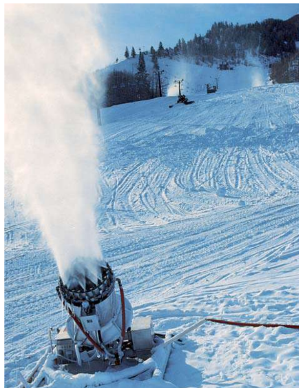
A snowmaking machine in operation.
