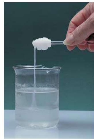
Figure 25.7 The nylon rope trick. Adding a solution of adipoyl chloride (an adipic acid derivative in which the OH groups have been replaced by Cl groups) in cyclohexane to an aqueous solution of hexamethylenediamine causes nylon to form at the interface of the two solutions, which do not mix. It can then be drawn off.
