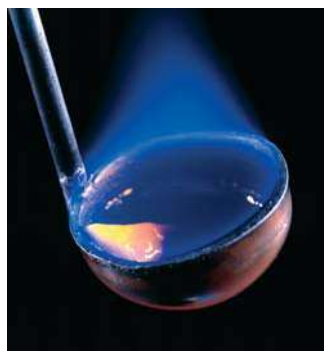
Sulfur burning in air to form SO 2 .
