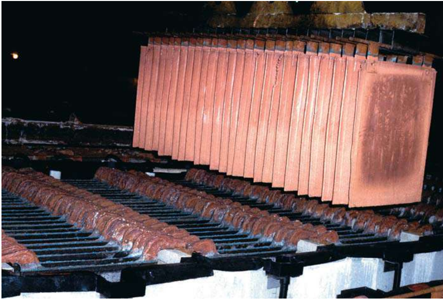
Figure 20.7 Copper cathodes used in the electrorefining process.
