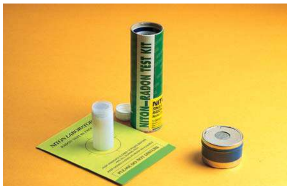
Figure 17.29 Home radon detectors: Long-term track etch (left) and short-term charcoal canister (right).
