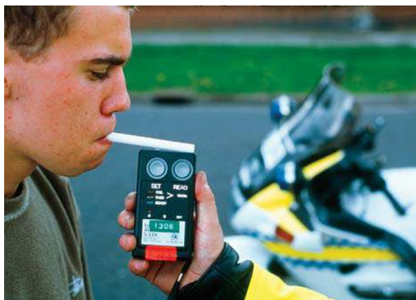
A driver being tested for blood alcohol content with a handheld breathalyzer.
