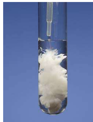
Figure 4.5 Formation of \text{BaSO}_4 precipitate.
