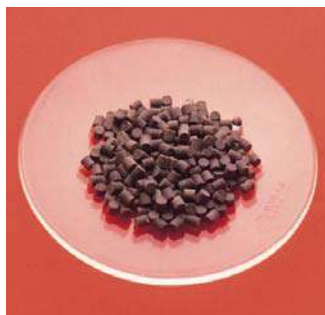
Platinum catalyst on alumina ( \text{Al}_2\text{O}_3 ) used in hydrogenation.
