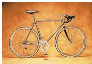
The frame of this bicycle is made of titanium.
