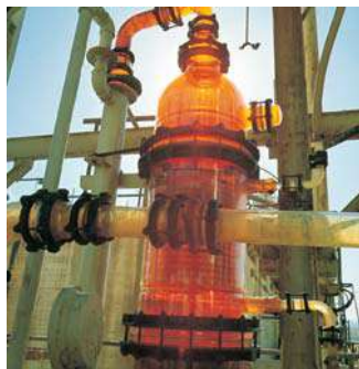
Figure 4.17 The industrial manufacture of bromine (a fuming red liquid) by oxidizing an aqueous solution containing \text{Br}^- ions with chlorine gas.
