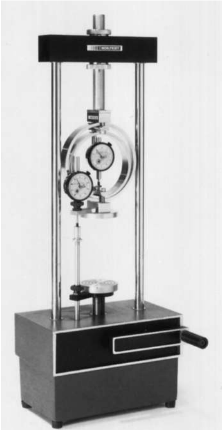
Figure 12.36 Unconfined compression test equipment (Courtesy of ELE International)
