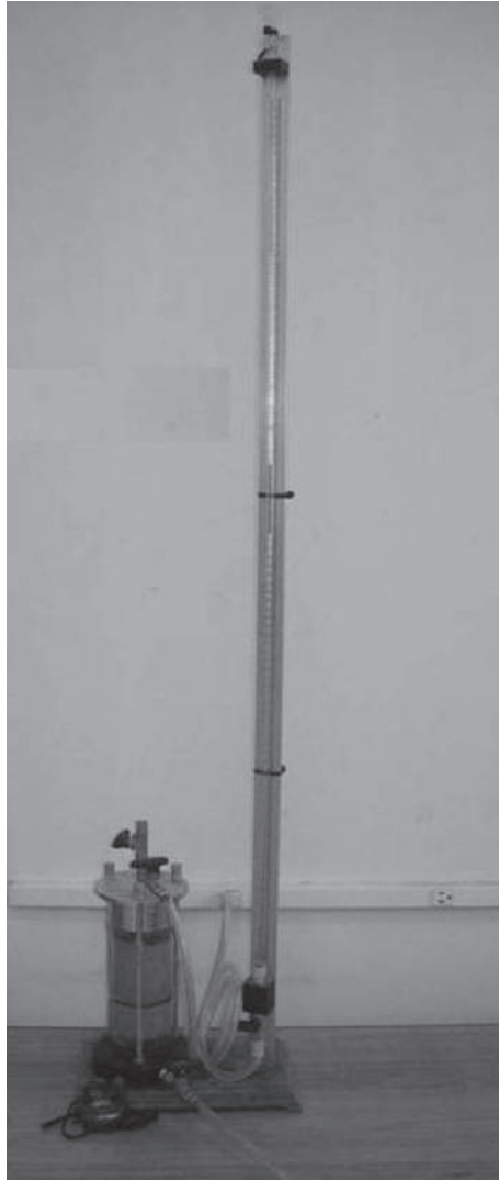
Figure 7.8 Falling-head hydraulic conductivity test arrangement for a granular soil in the laboratory (Courtesy of Khaled Sobhan, Florida Atlantic University, Boca Raton, Florida)
