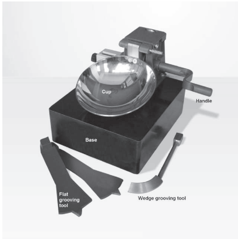
Figure 4.3 Liquid limit test device and grooving tools (Courtesy of N. Sivakugan, James Cook University, Australia)
