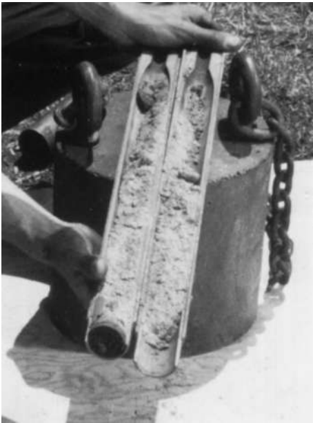
Figure 17.6 Split-spoon sampler, unassembled (Courtesy of ELE International)
