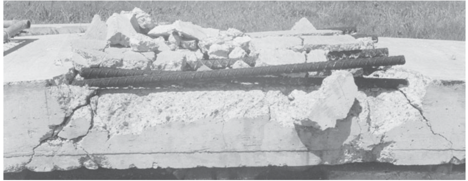
Fig. 8-38 Failure of a tension lap splice without stirrups enclosing the splice. (Photograph courtesy of J. G. MacGregor.)
